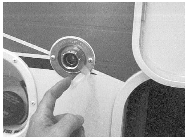
City Water Connection
