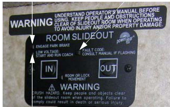
Low Voltage Indicator
