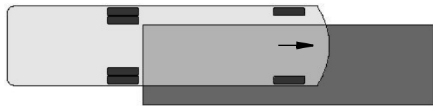
Weighing Right Front Corner
