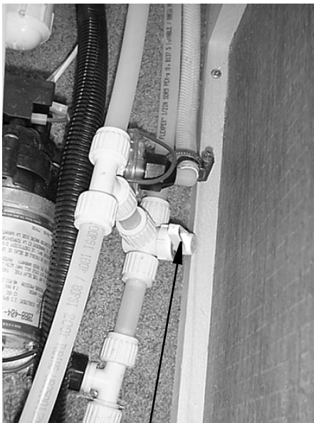
Waterline Drain Valve (Typical)
