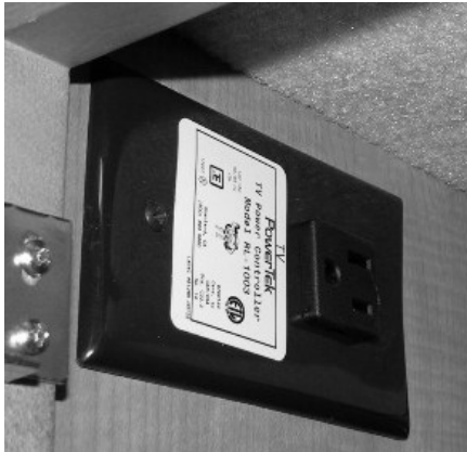
Front TV Ignition Switch Interlock -Typical View
