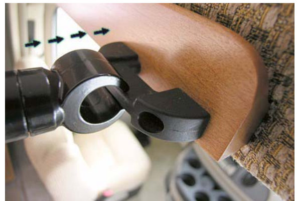
Attaching Bunk Ladder
