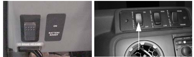
Battery Boost Switch
