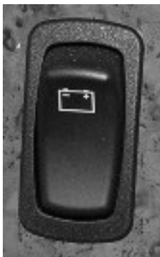
Battery Boost Switch (Located on dash)
