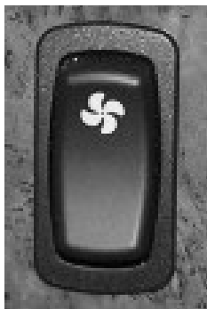
Defrost Fan Switch (Located on dash)
