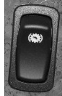
Grade Brake Switch (Located on dash)
