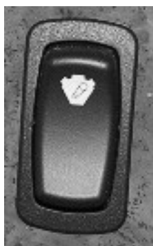
Overdrive Switch (Located on dash)
