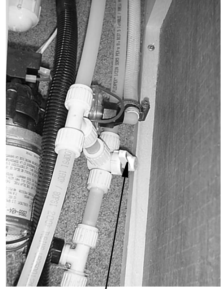
Waterline Drain Valve (Typical)
