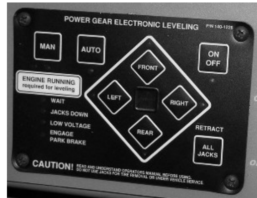
Leveling System Control Panel
