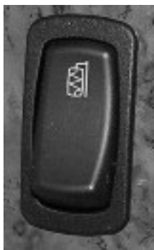
Mirror Heat Switch (Located on dash)
