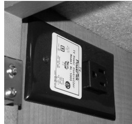
Front TV Ignition Switch Interlock -Typical View
