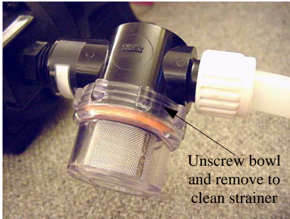
Water Pump Strainer -Typical View
