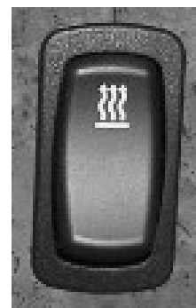
Coach Heat Switch (Located on dash)
