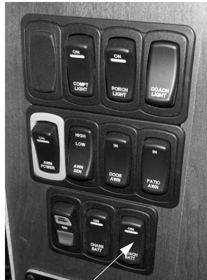
House/Coach Battery Disconnect Switch (Located near entrance door) -Typical View
