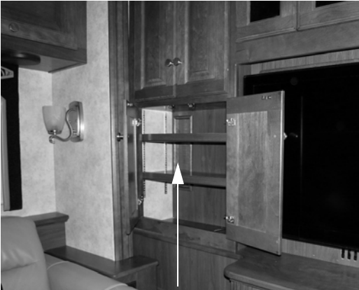
Water Supply Faucets (Located behind removable access panel in lounge area - remove shelving to access)
