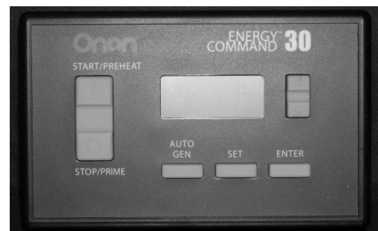
AGS Control Pad (Located near monitor panel)
