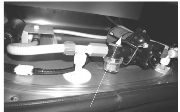
Water Pump (Located in driver side front compartment)
