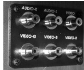
Audio Video Connection Plate -Typical View
