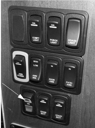
Entry Step Switch (Located near the entrance door) -Typical View
