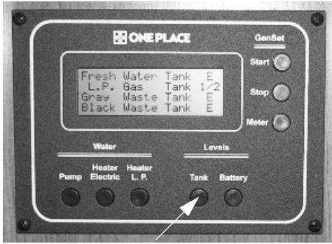
Tank Levels Switch
