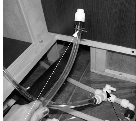
Antifreeze Siphon Tube • Insert into container of RV water system antifreeze.
