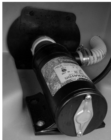
Waste Pump (Located underneath the rear driver side of coach) -Typical View
