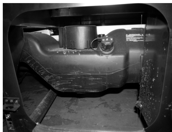
Diesel Exhaust Fluid Fill Tank (Located in passenger side compartment behind entrance door) -Typical View
