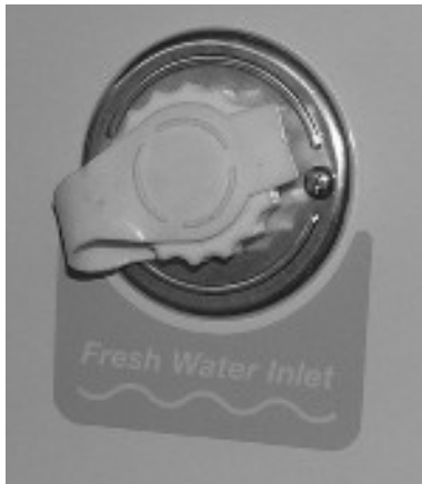
Fresh (City) Water Connection (located inside the exterior wash station)
