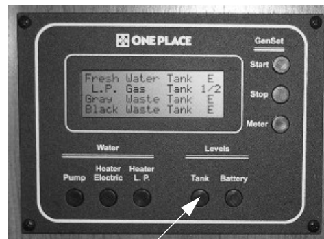
Tank Levels Switch
