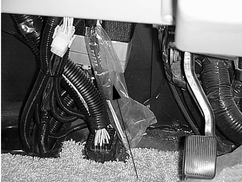
CB Power Wires (in plastic sheath)
