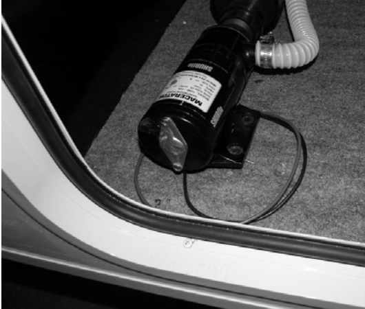
Waste Pump (Located in passenger side compartment ahead of rear axle) -Typical Installation
