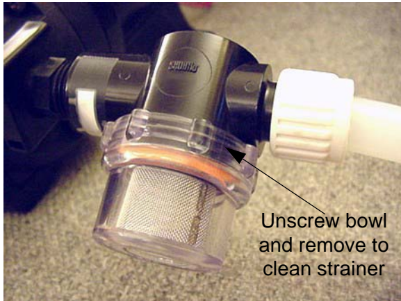
Water Pump Strainer -Typical View
