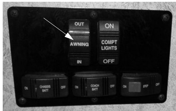
Awning Control Switch (Located near entrance door) -Typical View
