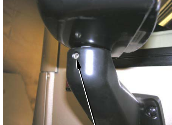
Mirror Head Pivot Lock Loosen Allen head set screw to pivot mirror head.* (Torque 75-100 in/lbs)
