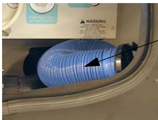
Sewage Drain Hose -Typical View
