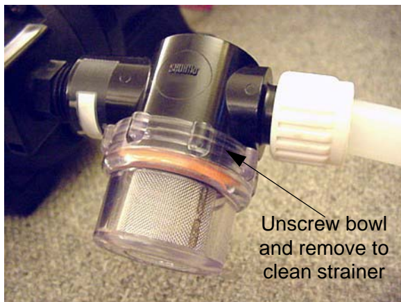
Water Pump Strainer -Typical View
