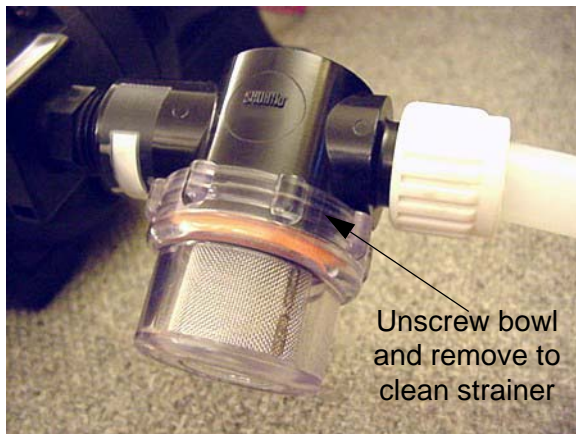
Water Pump Strainer -Typical View
