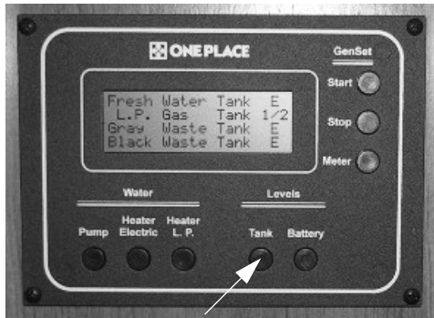
Tank Levels Switch
