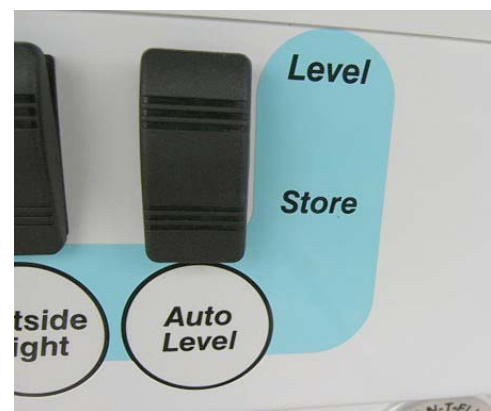
Auto Level Remote Switch (Located in exterior service center) -Typical View
