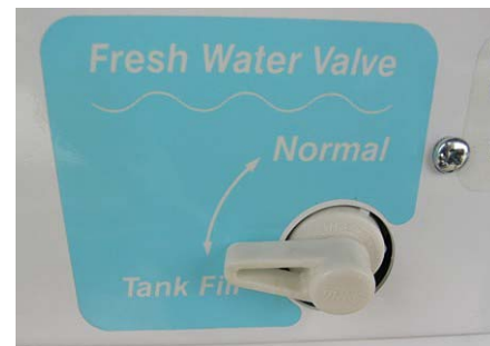
Fresh Water Valve in Tank Fill position (located inside the exterior wash station)
