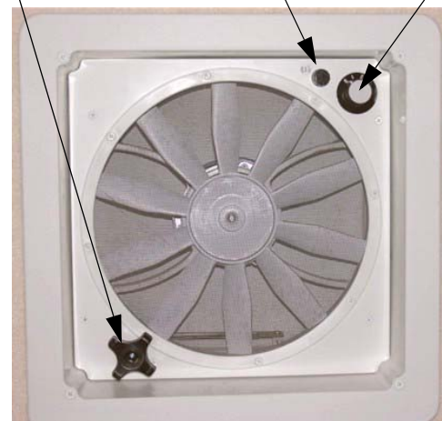
Power Roof Ventilator
