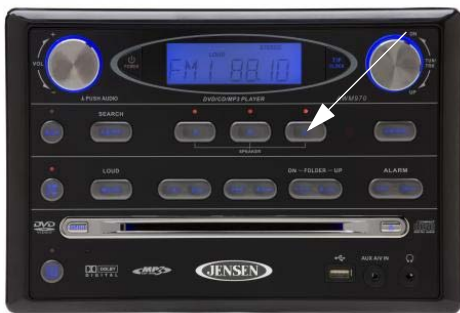
Exterior Speaker Switch “Speaker C” (Located on the interior DVD/CD/MP3/ AM-FM Stereo Radio)
