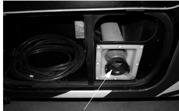
Sewage Drain Hose (Located in utility compartment)
