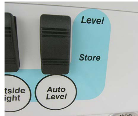
Auto Level Remote Switch (Located in the utility compartment) -Typical View
