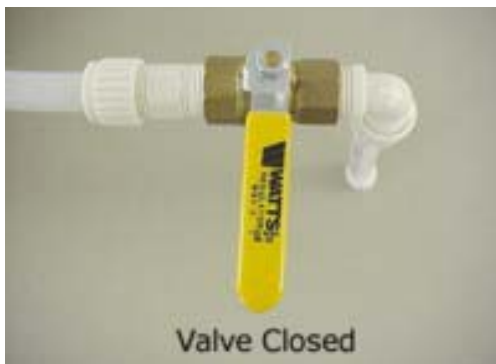
Water Tank Drain Valve (Located in first passenger side compartment) -Typical installation shown
