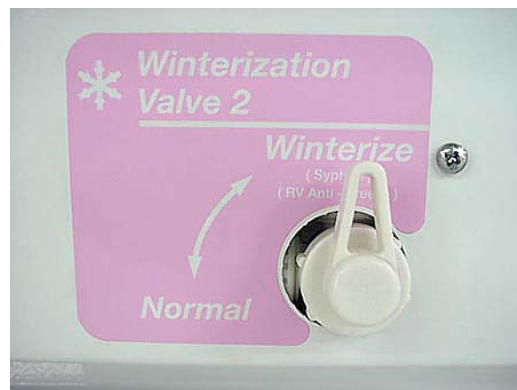
Winterization Valve 2 (See “Water System Drain Valve Locations” chart at the end of this section for location on your coach)
