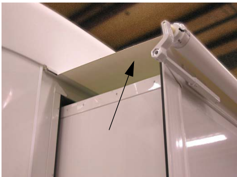
Slideout Cover-Awning -Typical View
