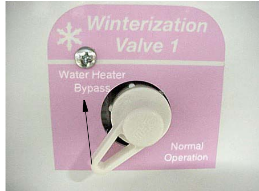
Winterization Valve 1 (See “Water System Drain Valve Locations” chart at the end of this section for location on your coach)
