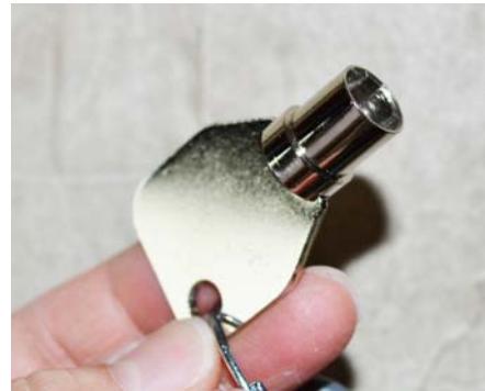
House/Coach Battery Access Cover Lock Key (Located on key ring)
