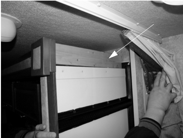
Slideout Travel Support -Typical installation shown
