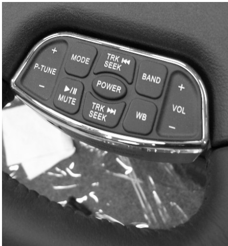
Steering Wheel Radio Remote Control
