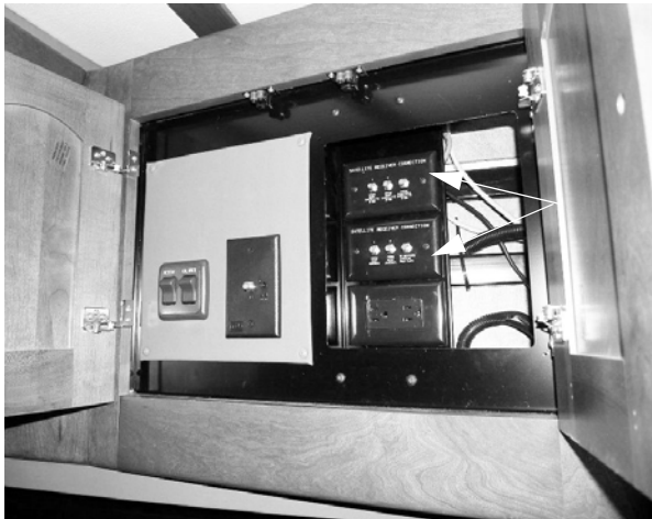
Interior Connections for Satellite Dish (Located in the overhead compartment above entrance door)
