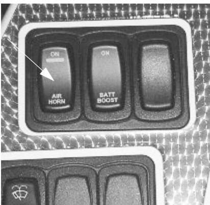
Air Horn Switch (Located on dash) -Typical View
