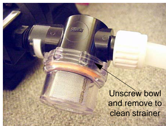
Water Pump Strainer -Typical View
