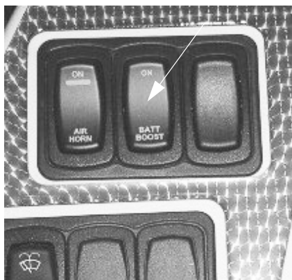
Battery Boost Switch (Located on dash) -Typical View
