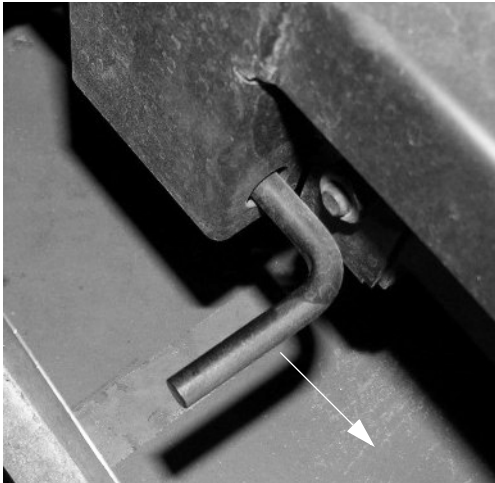
Release Lever (Located underneath the passenger side front hood)
