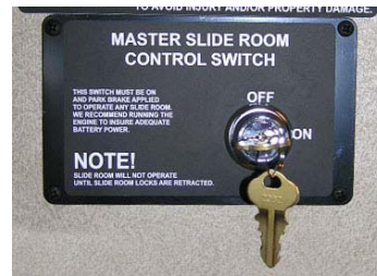
Slideout Room Keylock
