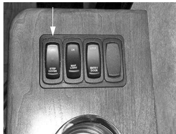
Step Cover Switch (Located on passenger side armrest) -Typical View
