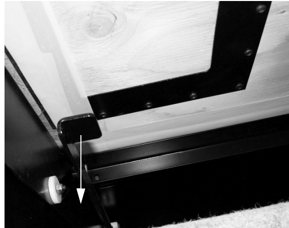
Emergency Retract Lever (Located underneath stepwell cover)
