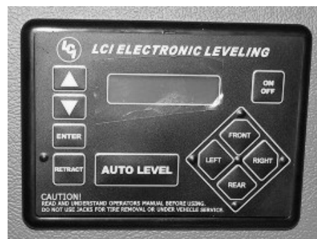
Leveling System Control Panel (Located on the driver side trim panel)
