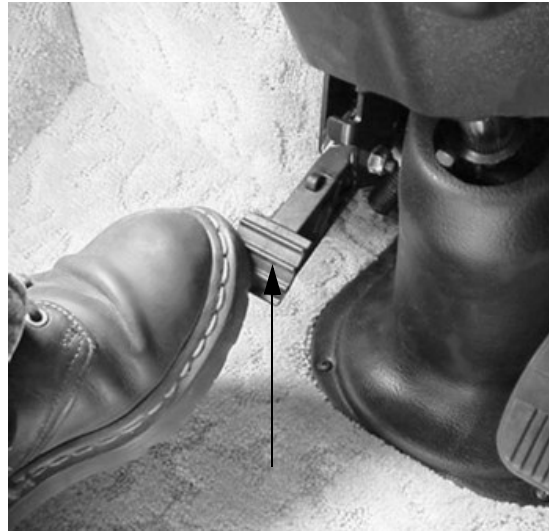
Press pedal to adjust steering wheel tilt or telescope
