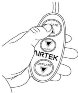
Air Mattress Hand Control (Located on inboard side of sofa arm)
