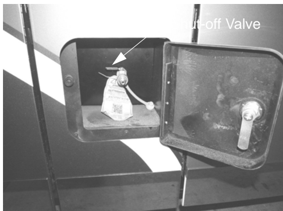
LP Accessory Connection (Located behind lockable access door on passenger side of coach) -Typical View
