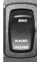
Radio Power Switch (Located on dash)
