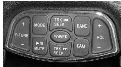
Steering Wheel Radio Remote Control
