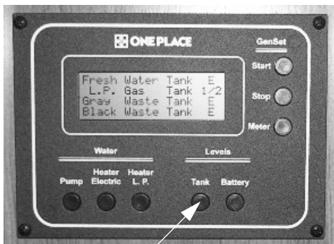
Tank Levels Switch
