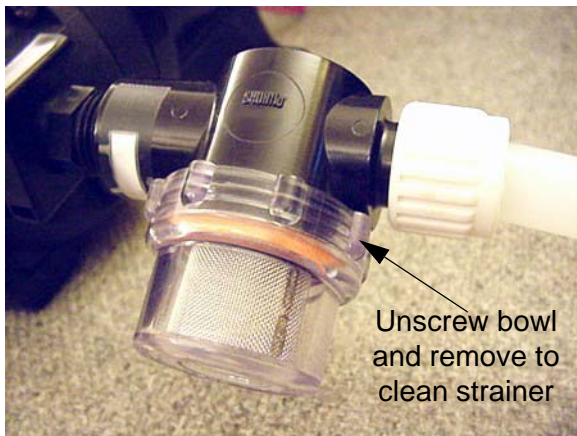
Water Pump Strainer -Typical View
