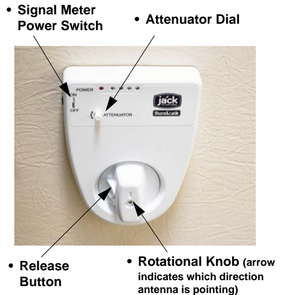
Digital Antenna Signal Meter (Located on ceiling)
