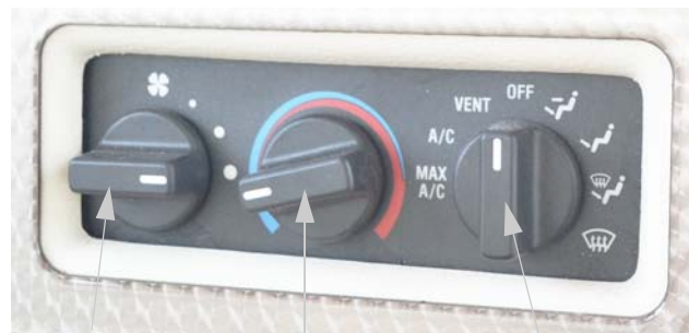
Blower Control Temp Control Mode Selector
