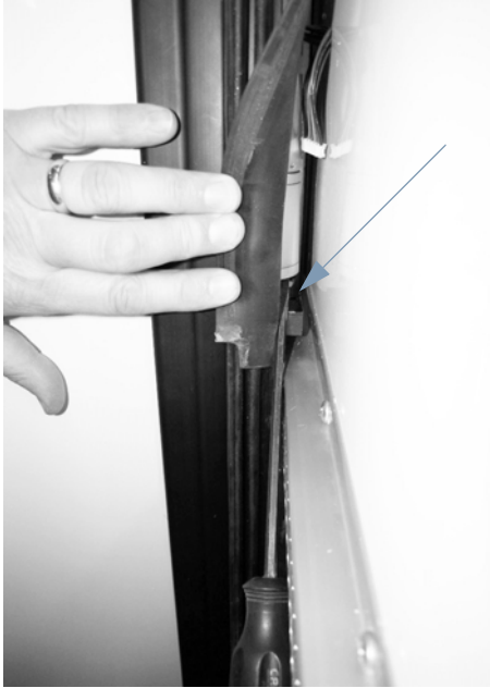
Slideout Motor (Located behind slideout wipe seal) • Use a screwdriver to push slideout motor UP (disengage).
