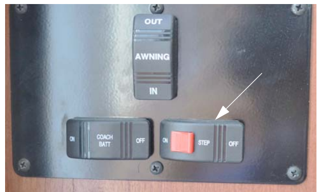
Entry Step Switch (Located near entrance door) -Typical View
