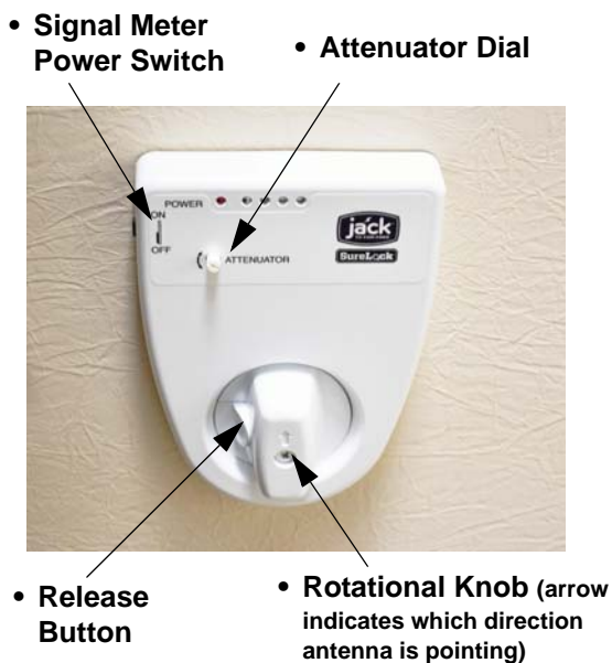
Digital Antenna Signal Meter (Located on ceiling)
