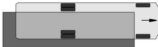
Weighing Right Rear Corner
