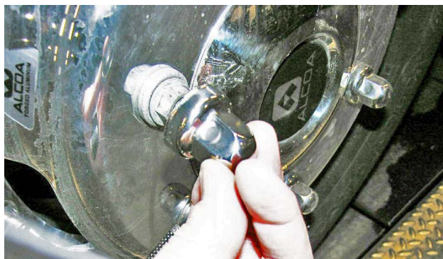
Remove the push on nut covers.
