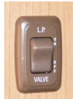
LP Tank Valve Switch
