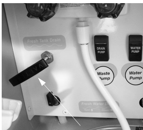
Water Tank Drain Valve -Typical View
