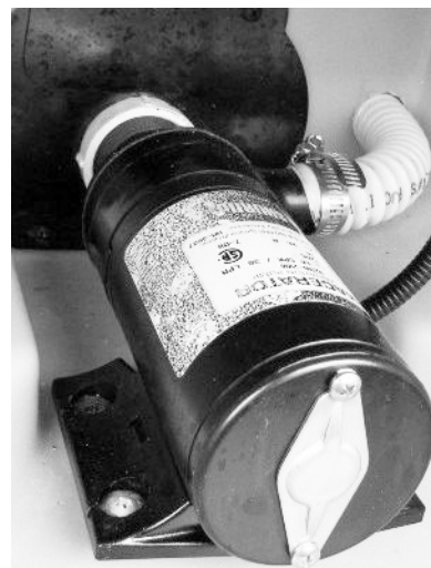
Waste Pump (Located beneath coach) -Typical View
