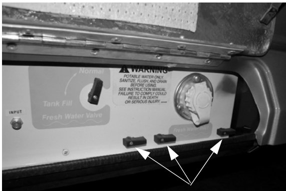
Waterline Drain Valves -Typical installation shown (See the "Water System Drain Valve Locations" chart at the end of this section for locations on your model)
