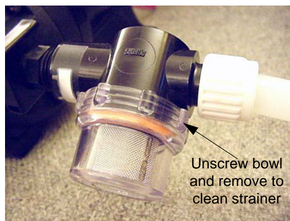
Water Pump Strainer -Typical View
