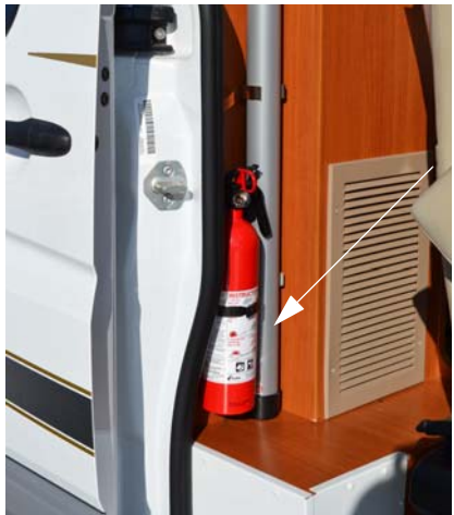
Fire Extinguisher (Located near sliding entrance door) -Typical installation shown
