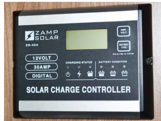
Solar Charge Controller (Located near monitor panel or in an exterior compartment, depending on model)
