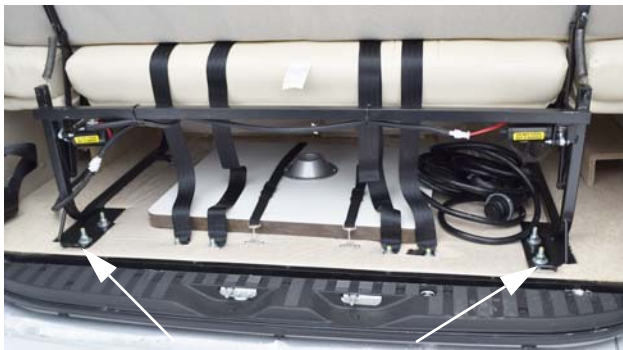
Tether Anchor Loop (Located on each end of sofa) - Open rear doors to access
