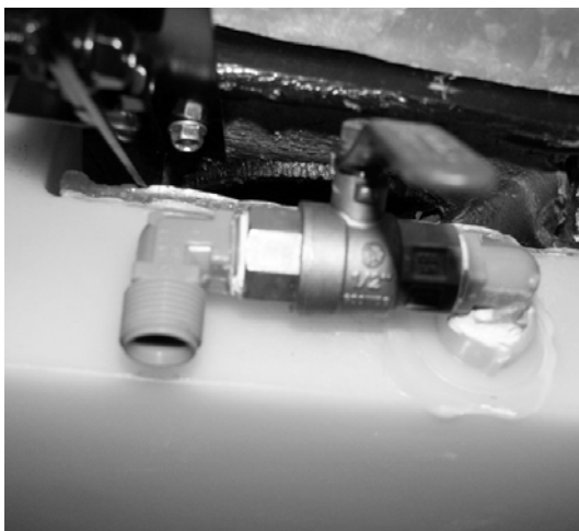
Water Tank Drain Valve (Located beneath running board, behind front passenger side door) -Typical installation shown
