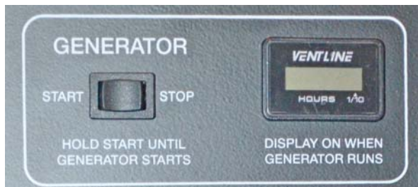
Generator Switch and Hourmeter on monitor panel
