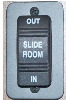
Slideout Switch -Typical View
