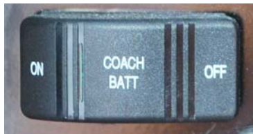
House/Coach Battery Disconnect Switch
