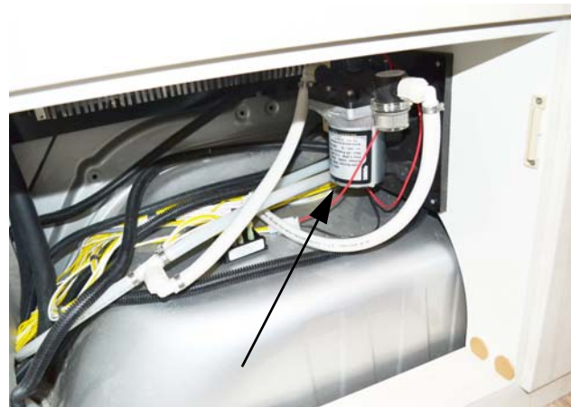
Water Pump (Located behind cabinet door below wardrobe)
