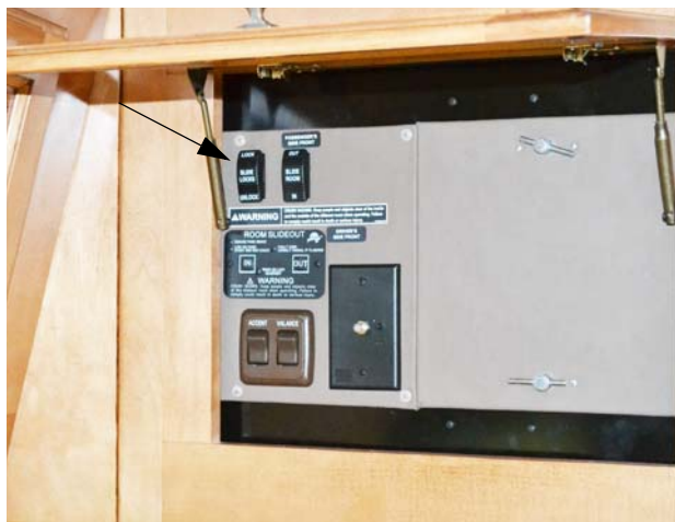
Slideout Room Travel Locks (Your model may be equipped with one or more types) -Typical View
