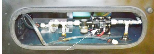
Water Pump (Located in driver side front compartment) -Typical installation shown
