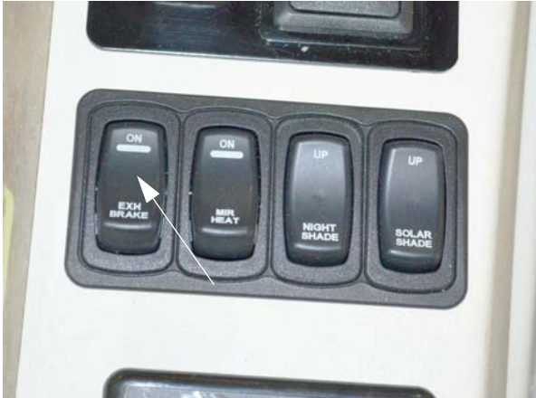
Exhaust Brake Switch (Located on driver side trim panel) -Typical View
