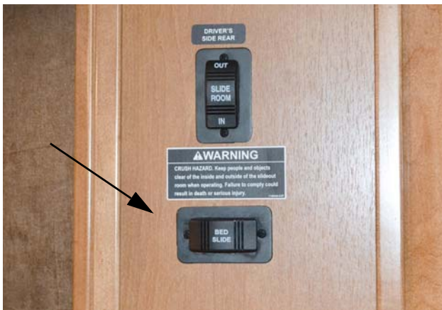
Bed Slide Control Switch (Located on forward bedroom wall) -Typical View
