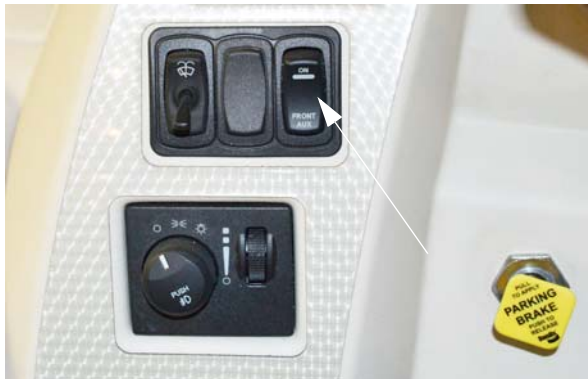
Front AUX Switch (Located on dash) -Typical View
