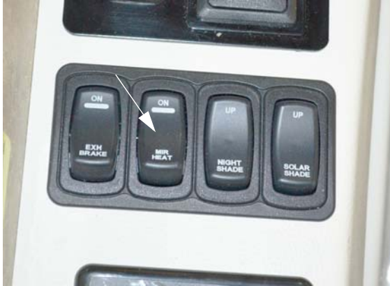
Mirror Heat Switch (Located on driver side trim panel) -Typical View
