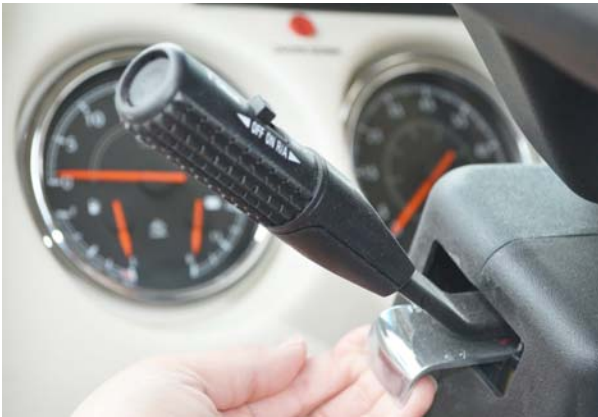
Hazard Warning Flashers (Typical View - your coach may differ depending on model)
