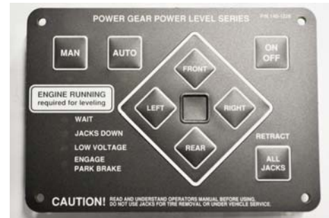
Leveling System Control Panel (Located on the driver side lower dash.)
