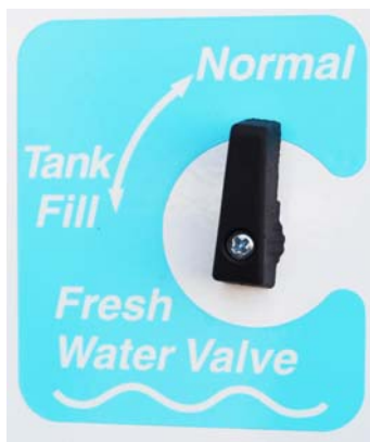
Fresh Water Valve (Located in water service center) -Typical View
