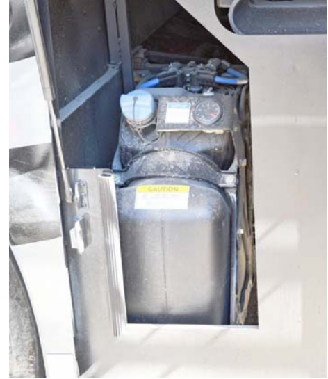
Diesel Exhaust Fluid Fill Tank (Located in driver side compartment behind rear wheel, depending on model) -Typical View
