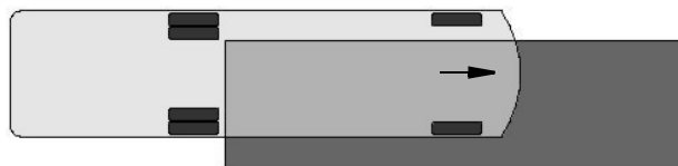
Weighing Right Front Corner
