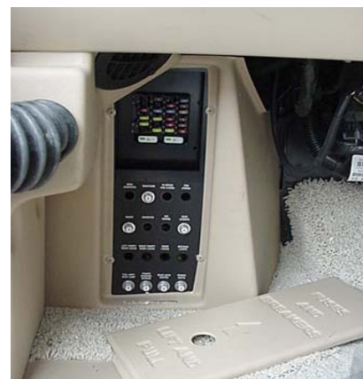
Automotive 12-Volt Circuit Breakers and Fuses (Located beneath left end of dash) -Typical View
