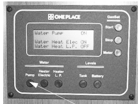
Water Pump Switch
