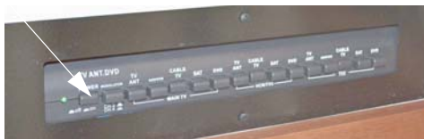
TV Signal Amplifier Switch (Located on Video Selection System)
