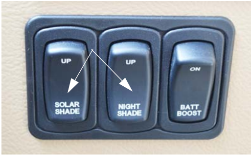
12-Volt Front Drop-Down Solar/ Night Shade Switches (Located on dash) -Typical View
