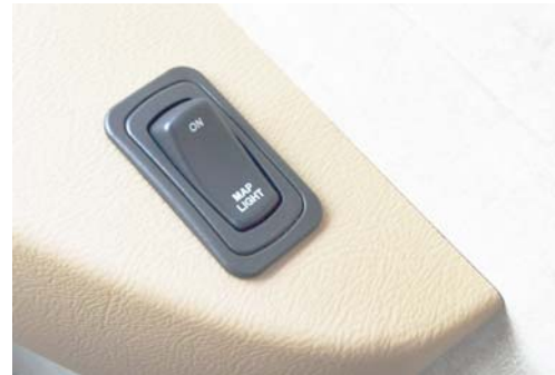
Passenger Side Map Light Switch (Located on passenger side trim panel)
