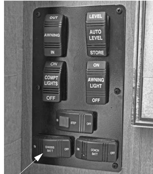
Chassis Battery Disconnect Switch (Located near entrance door) -Typical View
