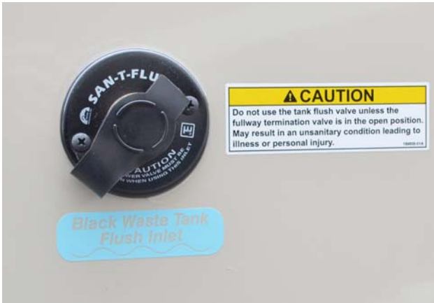
Black Waste Tank Flush Inlet (Located on left sidewall) -Typical View
