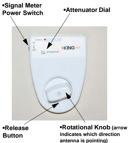
Digital Antenna Signal Meter (Located on ceiling)
