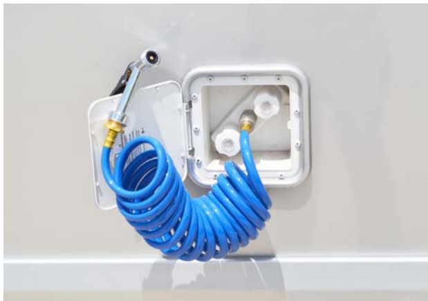
Exterior Shower/Wash Station (Typical)
