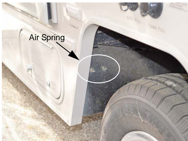
Rear Air Spring Valves (Located inside left rear wheel well -Typical View
