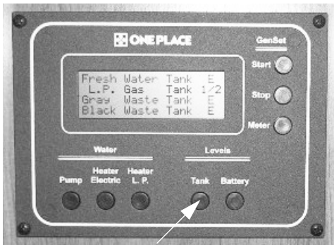
Tank Levels Switch
