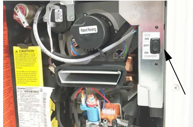
Water Heater Mode Switch (Located behind water heater access panel on exterior of coach)
