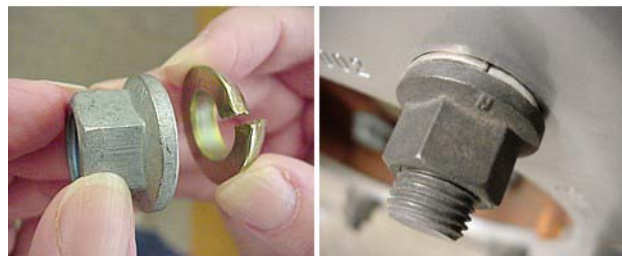
Steel Wheel Lug Nut and Washer (Hex Flange Nut with Split Cone Washer)
