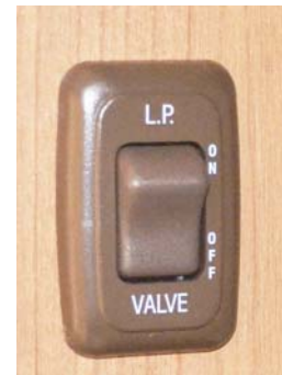
LP Tank Valve Switch
