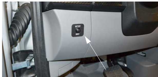
Battery Boost Switch (Located on lower driver side dash)
