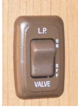
LP Tank Valve Switch
