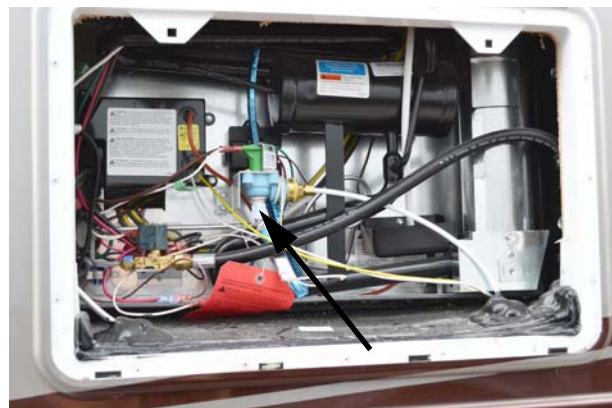
Ice Maker Water Supply Connection -Typical View
