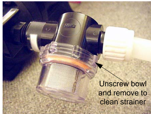
Water Pump Strainer -Typical View
