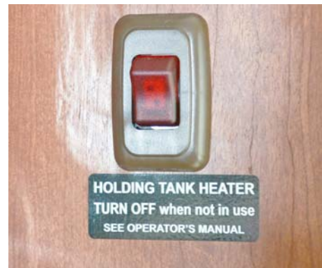
Holding Tank Heater Switch (Located near monitor panel) -Typical View
