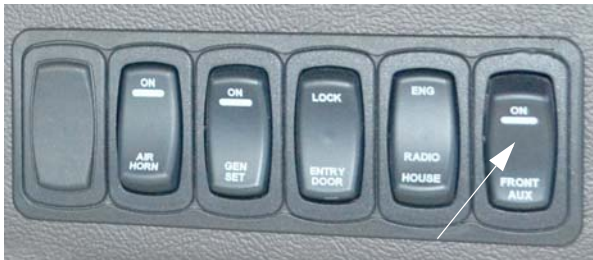
Front AUX Switch (Located on dash) -Typical View
