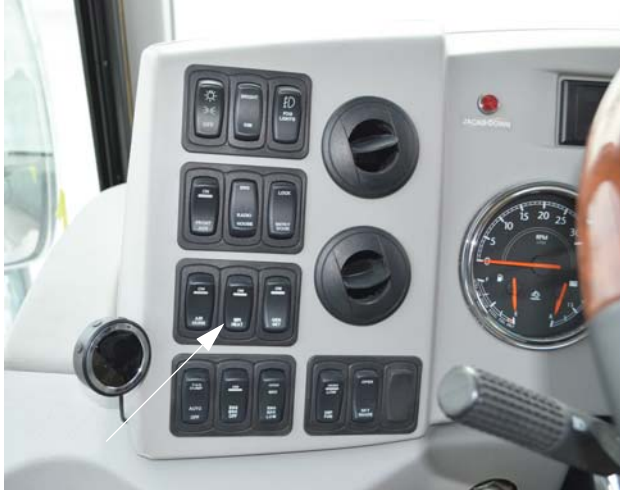
Mirror Heater Switch (Located on dash) -Typical View
