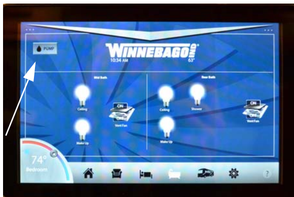
Water Pump Switch (Located on touch tablet "Bath" screen) -If Equipped Tap to turn Water Pump ON/OFF. • White text indicates ON • Black text indicates OFF
