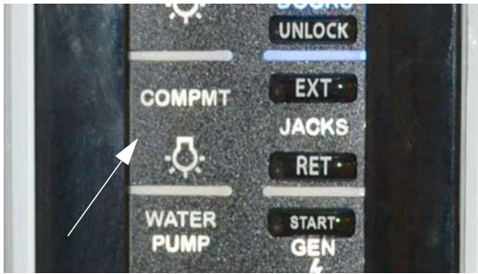
Compartment Lights Switch (Located near entrance door and/or inside a driver side compartment) -Typical View
