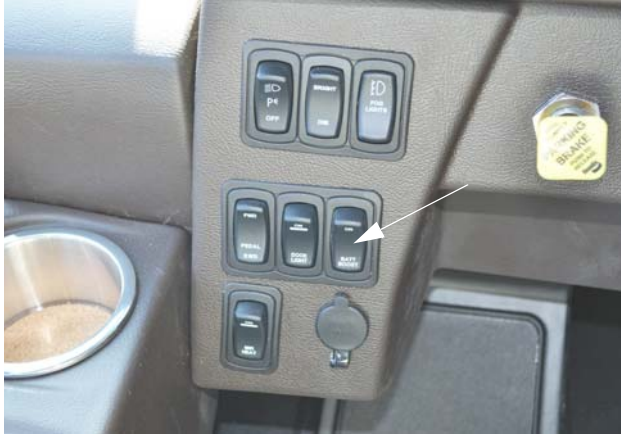
Battery Boost Switch (Located on dash)
