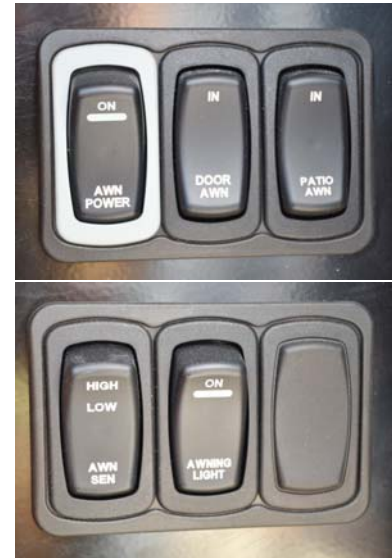
Power Awning Control Switches (Located near the entrance door) -Typical View
