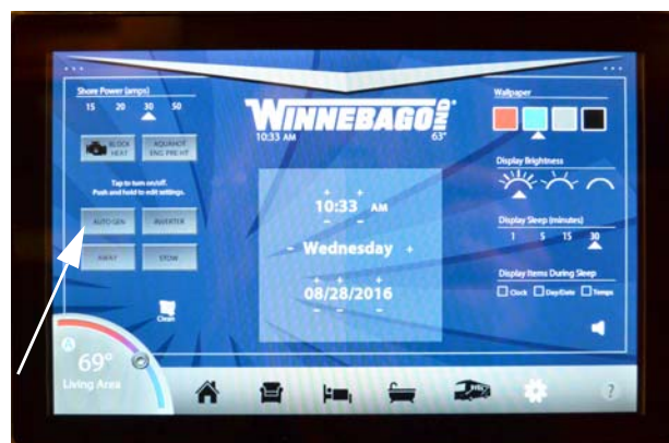
Generator Switch (Located on touch tablet "Utilities" screen)
