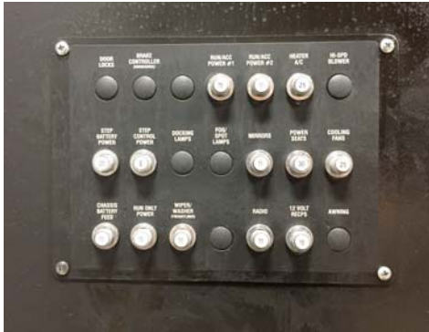
Automotive Circuit Breakers (push to reset)
