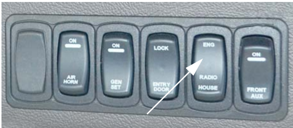
Radio Power Switch (Located on dash) -Typical View
