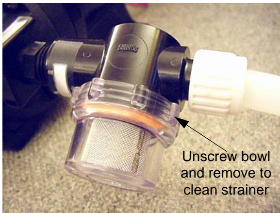
Water Pump Strainer -Typical View
