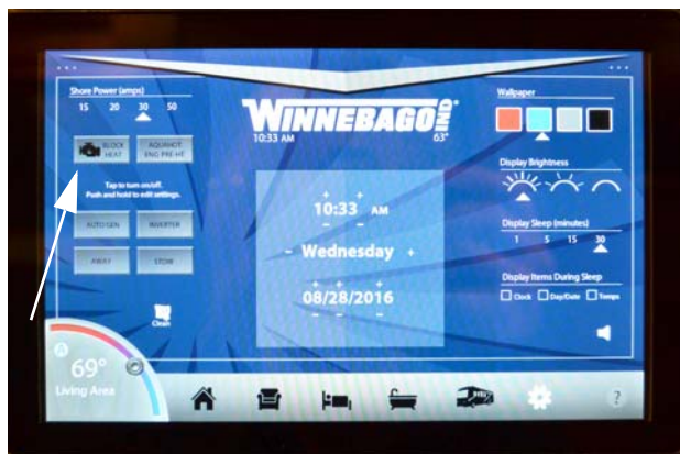
Diesel Engine Heater Switch
