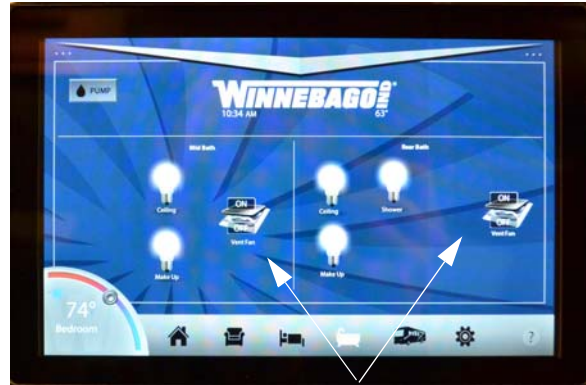
Power Roof Ventilator Switch (Located on touch tablet "Bath" screen) -If Equipped
