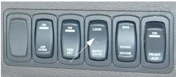
Power Door Locks - Entry Door (Located on dash) -Typical View
