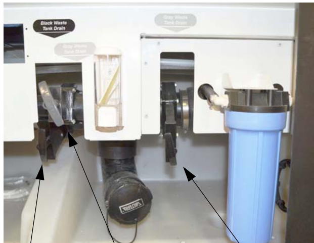
Black Waste Tank Drain Valve Gray Waste Tank Drain Valve #1 Gray Waste Tank Drain Valve #2
