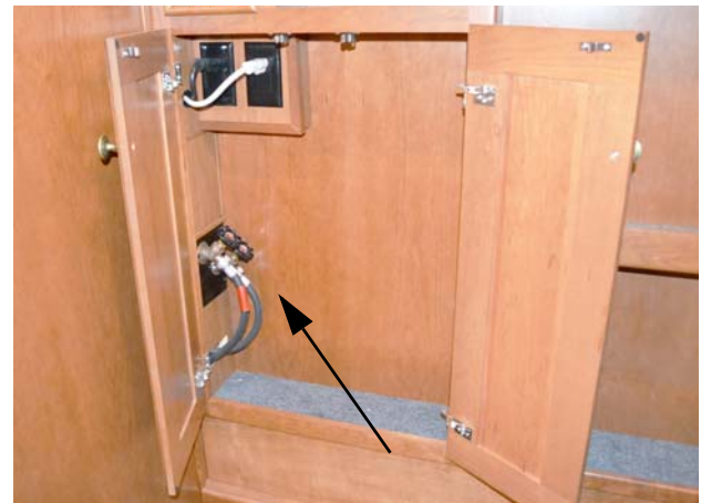
Water Supply Faucets (Located inside bathroom wardrobe cabinet) *Model 45RD
