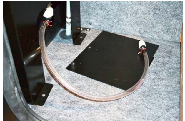
RV Antifreeze Siphon Tube (Located in the third compartment on passenger side of coach)
