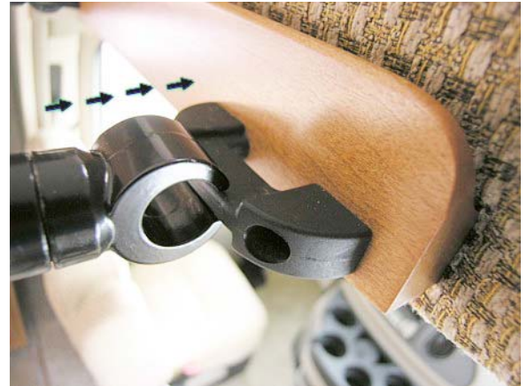
Attaching Bunk Ladder
