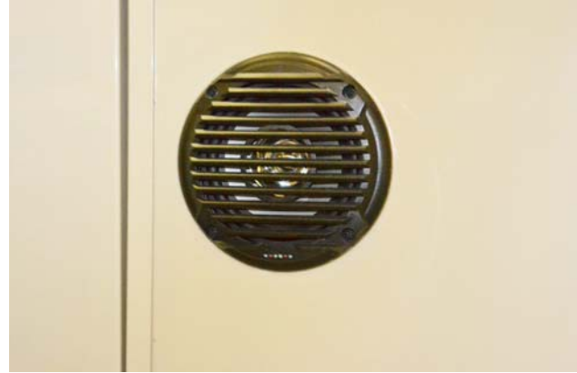
Exterior Speaker (Located on right sidewall) -Typical View
