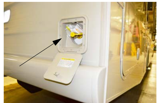
LP Accessory Connection (Located behind access door at the rear passenger side of the vehicle)
