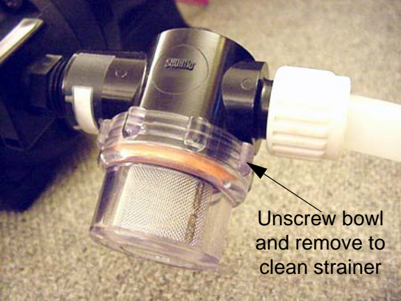
Water Pump Strainer -Typical View
