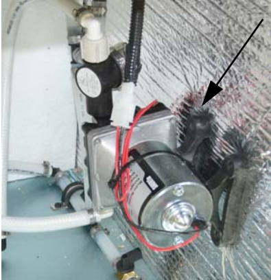
Water Pump (Located in passenger side compartment behind rear axle) *Model 26HE shown
