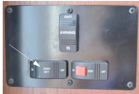
House/Coach Battery Disconnect Switch (Located near entrance door) -Typical View
