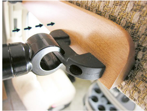
Attaching Bunk Ladder
