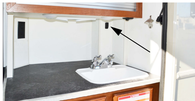
Sink Drain Pump Switch (Located near exterior sink) -Typical View
