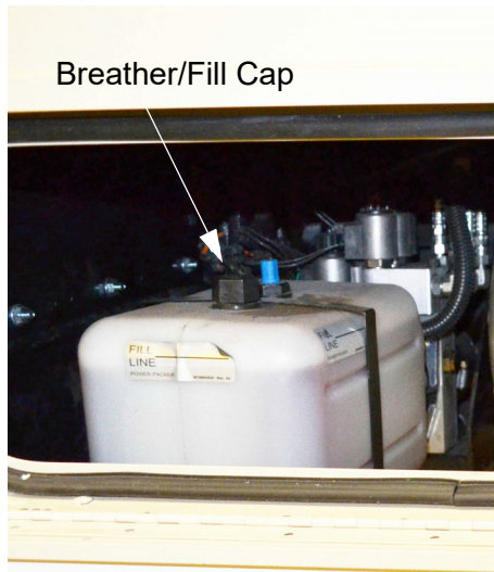
Hydraulic Oil Reservoir (Located behind driver side front tire) -Typical View
