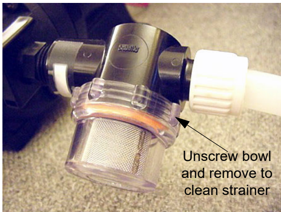
Water Pump Strainer -Typical View
