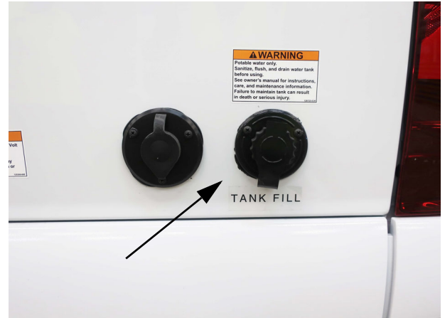
Tank Fill Inlet (Located on the left or right sidewall, depending on model) -Typical View
