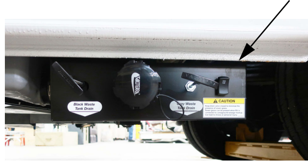
Waste Pump Switch (Located beneath motorhome near sewage drain outlet) -Typical View
