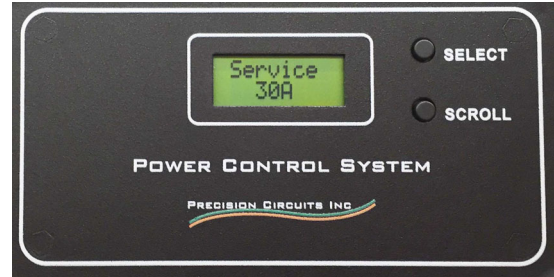
PCS Display Panel (Located near monitor panel) -Typical View
