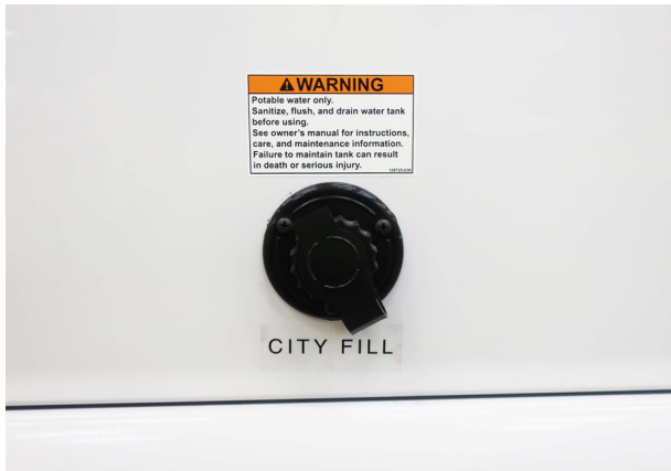
City Fill Inlet (Located on the left or right sidewall, depending on model) -Typical View
