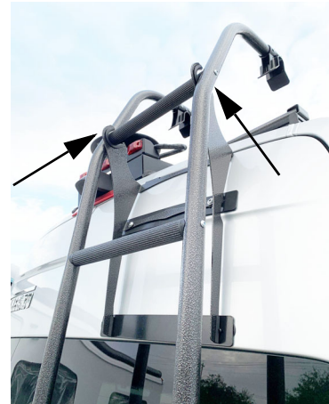
Ladder Storage Rungs -Typical View
