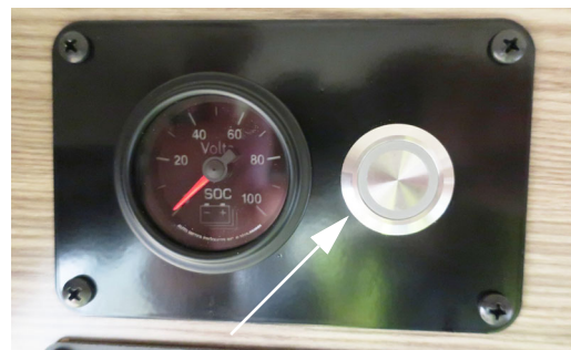
Pure 3 ON/OFF Button (Located on an interior cabinet) -Typical View
