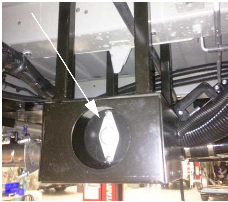
Waste Pump (Located beneath motorhome)
