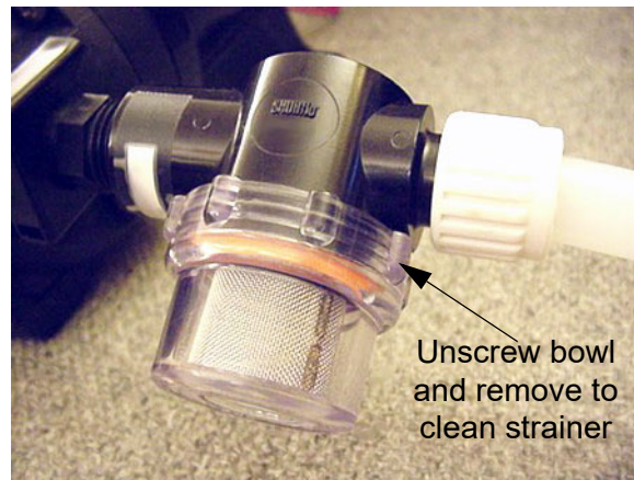
Water Pump Strainer -Typical View
