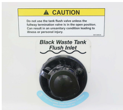
Black Waste Tank Flush Inlet (Located on right sidewall)
