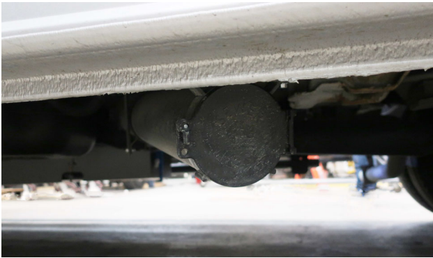
Sewage Drain Hose (Located on driver side front of rear wheel) -Typical View
