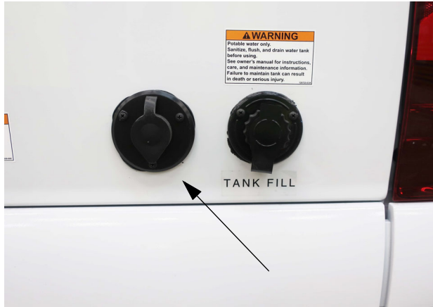
Cable TV Input Connection (Located on the left sidewall) *Model 70KL shown
