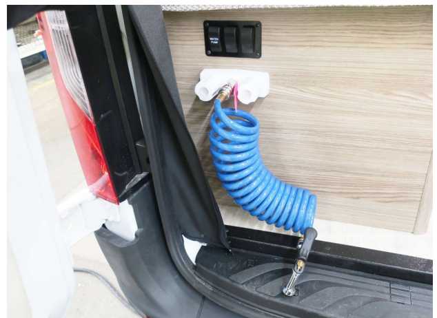
Exterior Shower/Wash Station (Located behind rear driver side door) *Model 70BL shown
