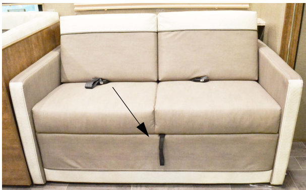
Security Latch Strap Pull strap DOWN to release security latch -Typical View
