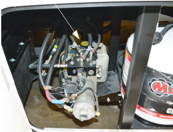
Hydraulic Oil Reservoir (Located behind driver side front tire) -Typical View
