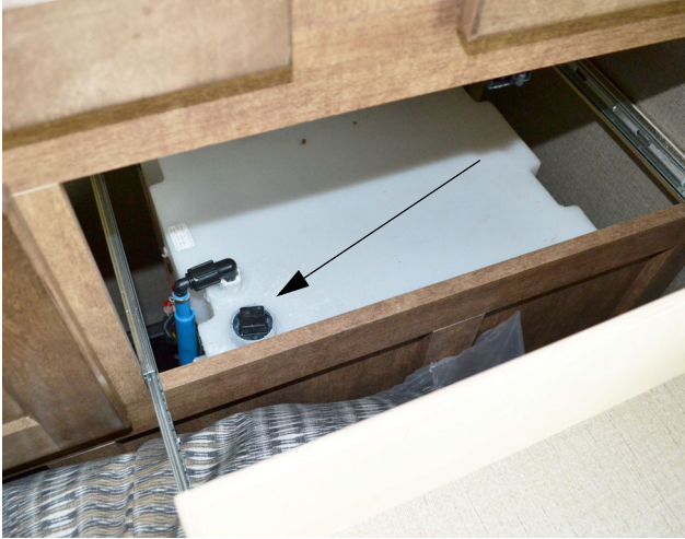
Water Tank Gravity Fill Access • Model 30R - Located in rear wardrobe. Remove top rear drawer to access.
