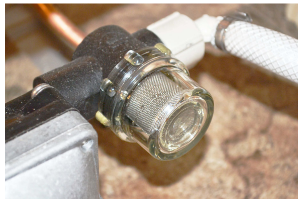
Exterior Sink Filter Screen (Located in the passenger side compartment behind rear axle) -Typical View
