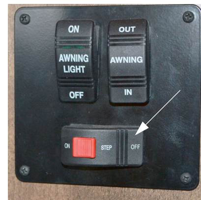
Entry Step Switch (Located near entrance door) -Typical View
