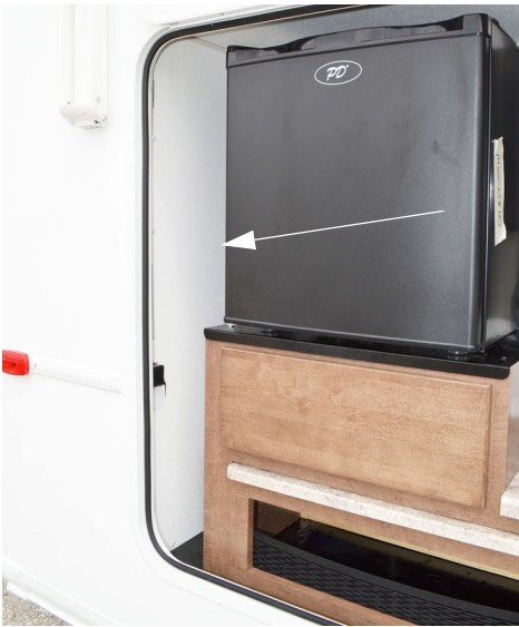
Water Tank Gravity Fill Access • Models 26M, 29L, 31P - Located rear of tailgate refrigerator. Remove screws on access panel.
