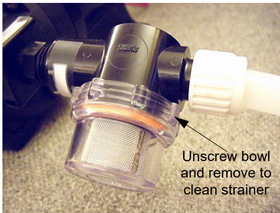
Water Pump Strainer -Typical View
