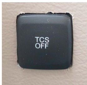
Traction Control Button is located left of the steering wheel. -Typical View
