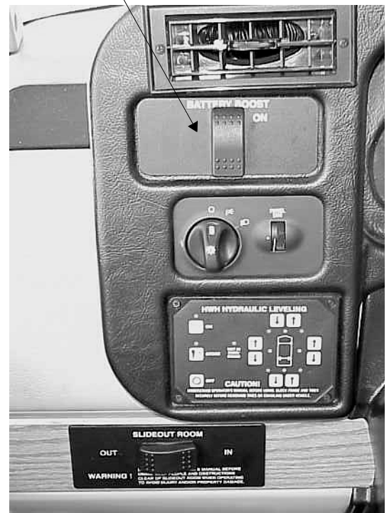
Battery Boost Switch
