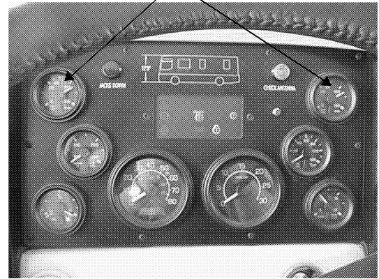
Air Pressure Gauges
