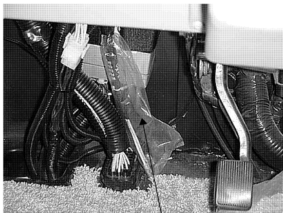
CB Wires (in plastic sheath)
