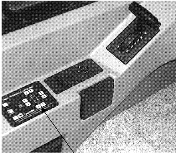
Leveling System Control Panel
