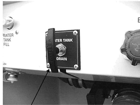
Water Tank Drain Valve (pull to open)
