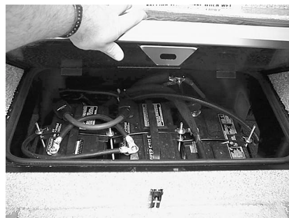
Remove step cover to access batteries
