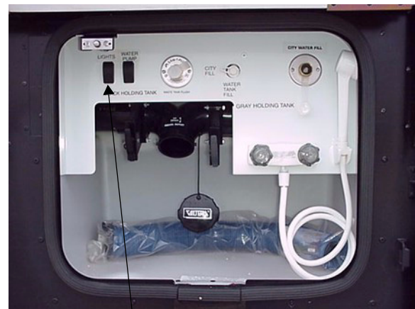
Utility Light Switch
