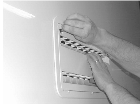
Turn latches open with coin
