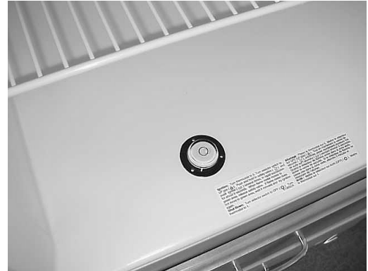
Place bubble level in bottom of refrigerator
