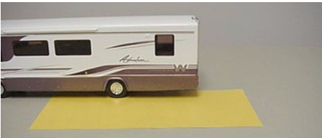
Weighing Left Rear 'Corner'
