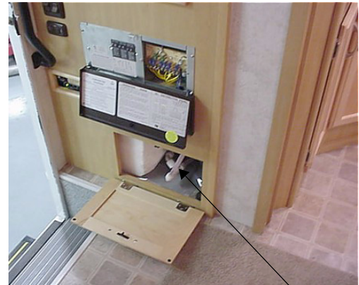
Water Heater Bypass Valve Location
