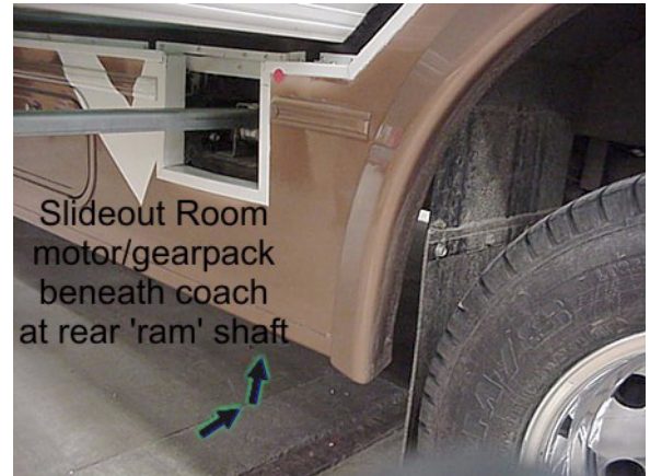
Slideout motor/gear location
