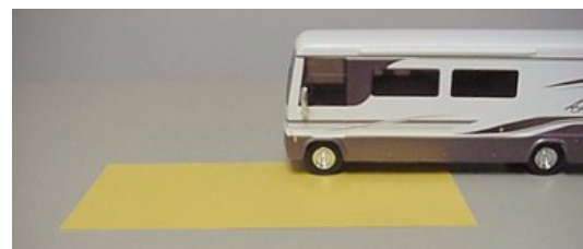
Weighing Left Front 'Corner'
