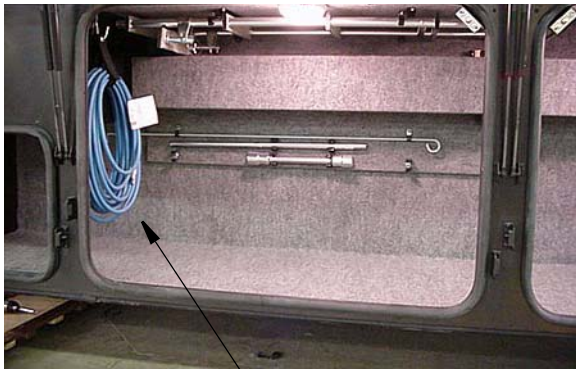
Air hose in exterior compartment
