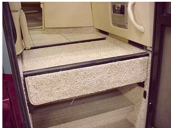
Step Cover shown in extended position
