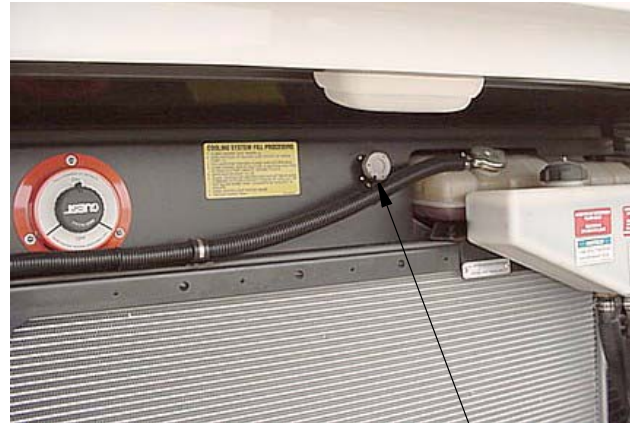
Diagnostic plug on rear engine compartment shroud
