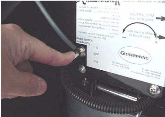
Press and hold switch to retract power cord reel (optional)
