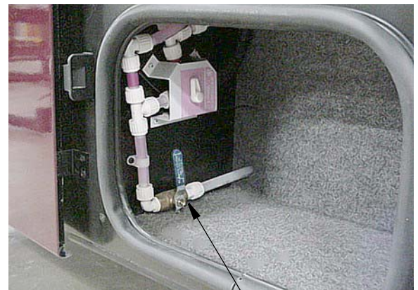
Water Line Drain Valve - additional model 40KD only (in RH rear storage/battery compartment)
