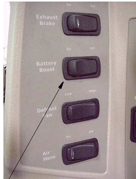
Battery Boost Switch
