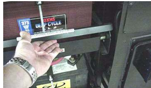
Lift Battery Tray Retainer Latches
