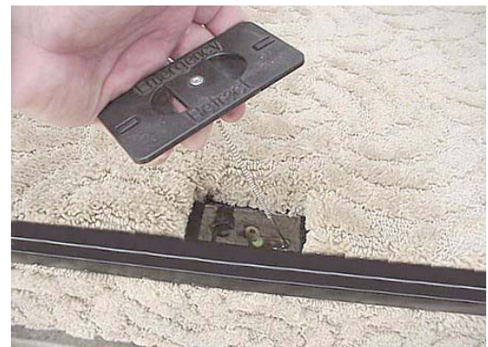
Pull chain to release step mechanism and manually slide step cover back.
