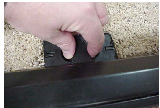
Lift snap-in plate from front edge of step cover.
