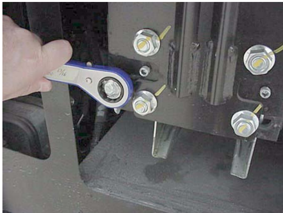
Crank the Slideout Retract Bolt with the Ratchet Wrench provided.
