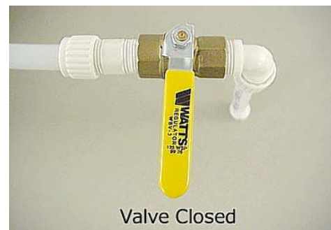
Water Line Drain Valve - additional model 40KD only (in RH rear storage/battery compartment)
