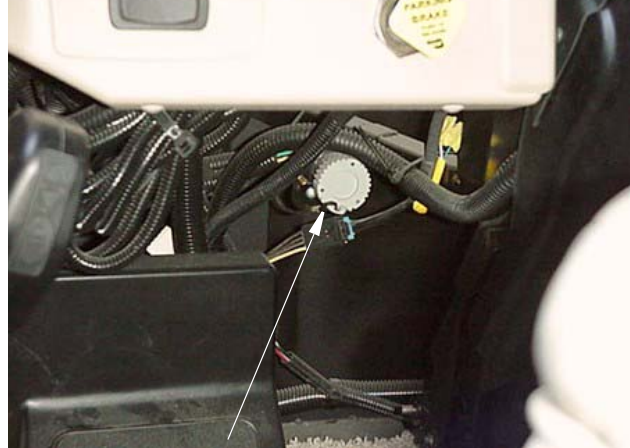
Diagnostic plug on steering column support beneath left side of dash
