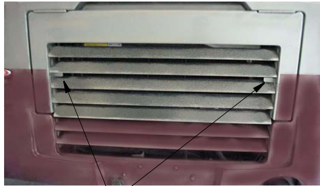
Lift latches and swing grille upward
