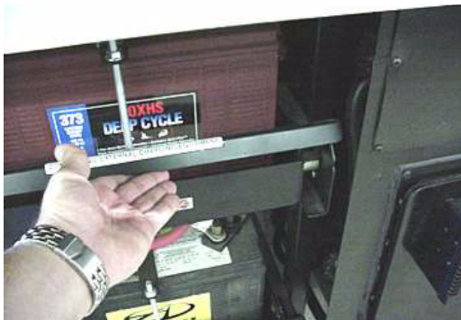
Lift Battery Tray Retainer Latches
