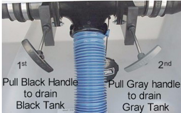
Holding Tank Valves (Typical)
