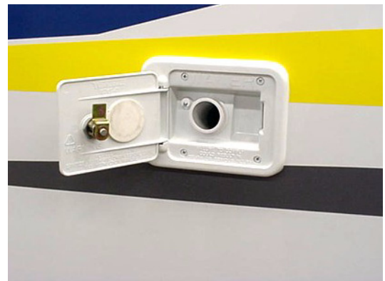
Water Tank Gravity Fill (typical)
