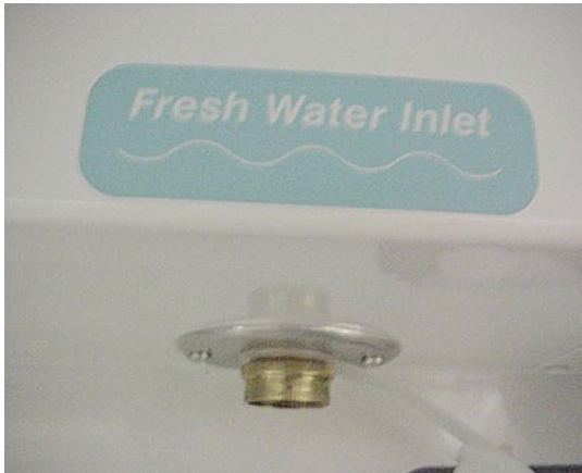
Fresh (City) Water Inlet
