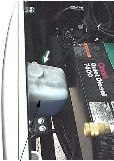
Windshield Washer Reservoir behind front "hood" panel.
