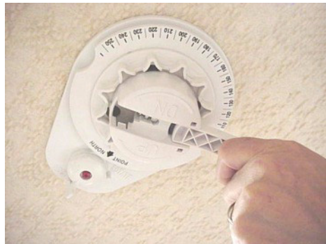
Digital Satellite Dish Control located on ceiling
