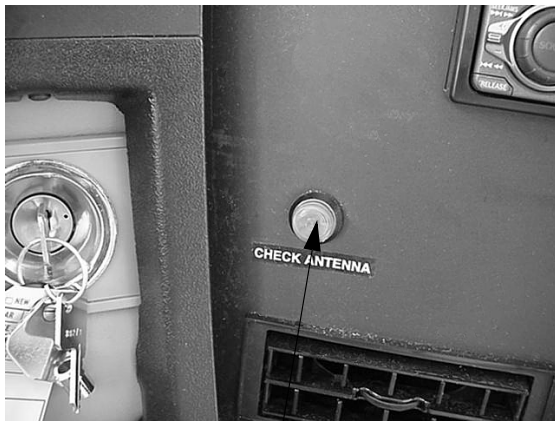
“Check Antenna” Light
