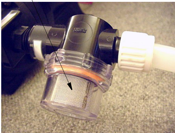
Water Pump Strainer
