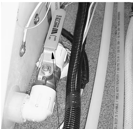
Water Tank Drain Valve (Typical) in water service center or passenger side exterior compartment
