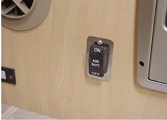
Aux. Batt. Switch (Near entrance door)
