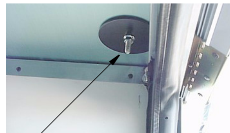
Model 430V Bolt is visible on ceiling of exterior storage compartment below dinette.
