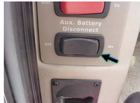
Aux. Batt. Switch (near entry step)
