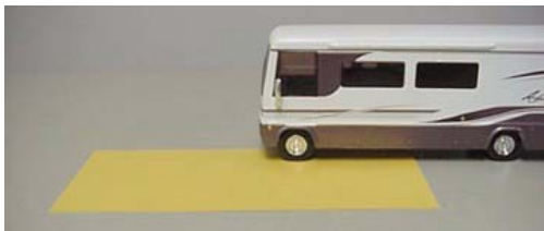
Weighing Left Front 'Corner'
