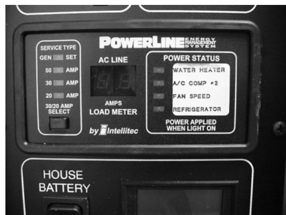
PowerLine EMS Display on OnePlace Monitor Panel
