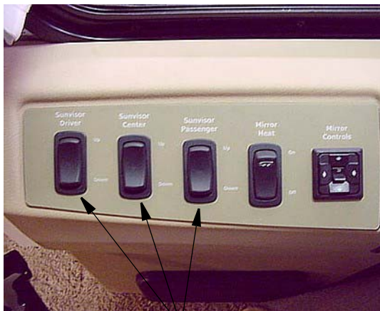
Driver Side Sunvisor Switches (center visor not equipped on model 40KD)
