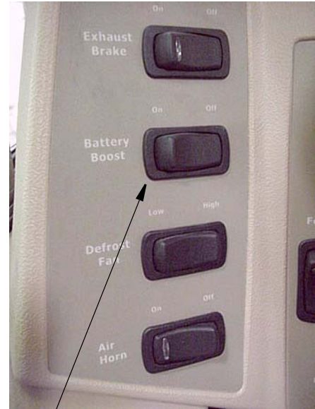
Battery Boost Switch
