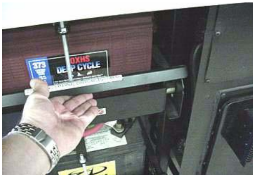
Lift Battery Tray Retainer Latches
