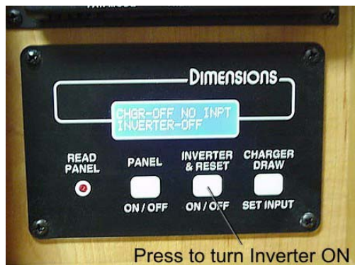
Inverter/Charger Control Panel
