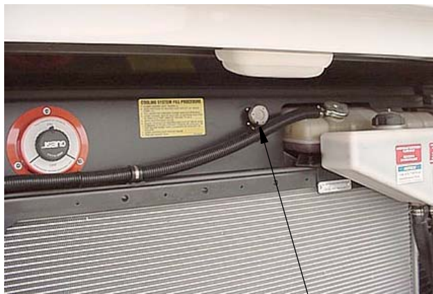
Diagnostic plug on rear engine compartment shroud
