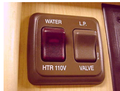
LP Tank Valve on OnePlace Panel
