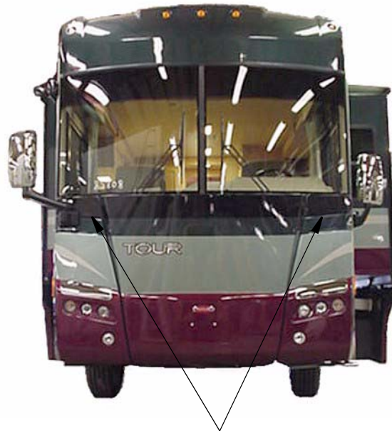
Cowl Panels Use care when cleaning to maintain high-gloss finish. See "Plastic Parts- Cleaning"
