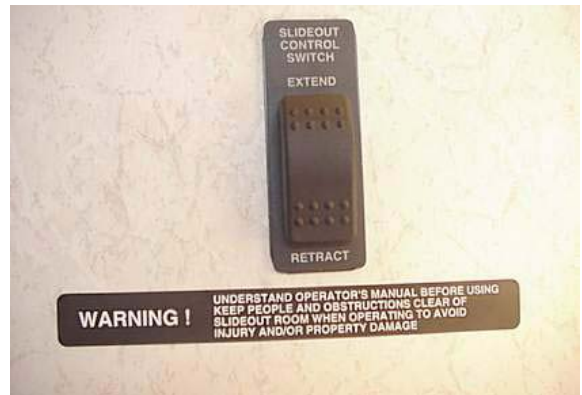
Rear Slideout Switch (on wall in rear of couch - varies by model)
