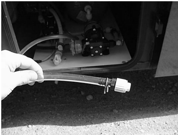
RV Antifreeze Draw Tube in water center or near water pump (insert into container of RV water system antifreeze)
