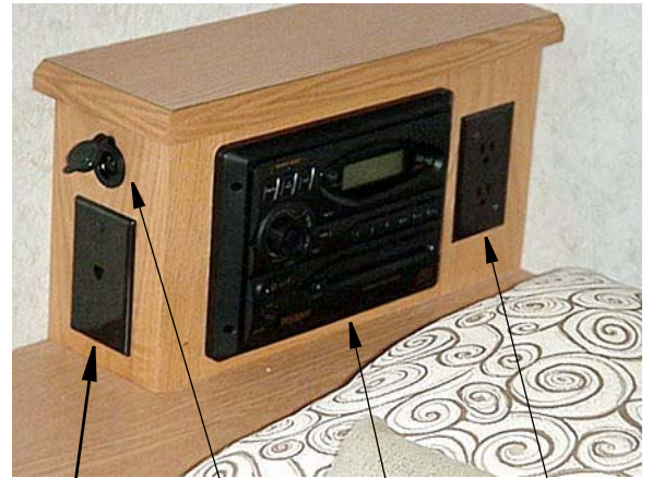
Bedroom Radio Rear Phone Jack 12-volt DC Electrical Outlet AC Electrical Outlet
