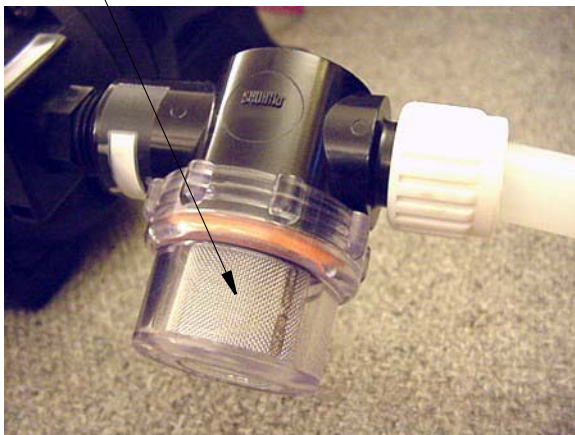
Water Pump Strainer
