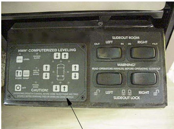
Leveling System Control Panel (tip-out panel on lower right dash)
