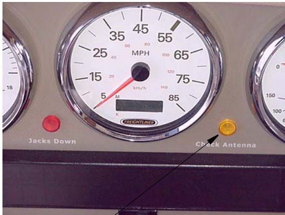
"Check Antenna" Light
