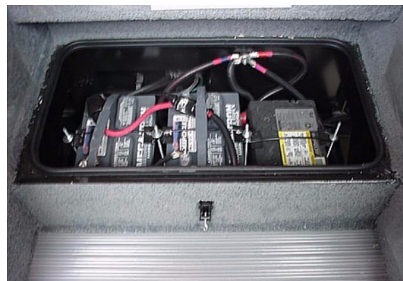
Release latch and lift step to access house and chassis batteries
