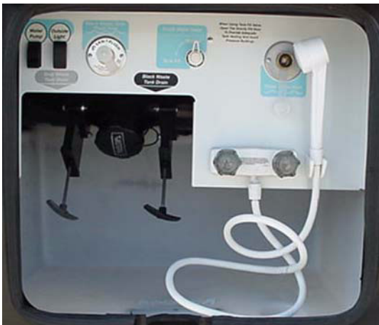
Water Service Center
