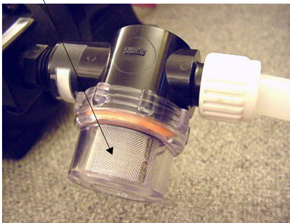
Water Pump Strainer
