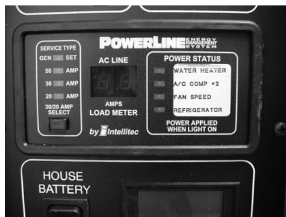
EMS Display on Monitor Panel -Typical View
