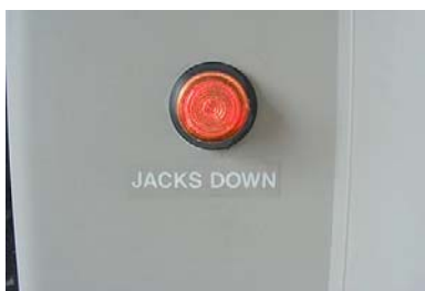
“Jacks Down” Light on Dash (Typical View)
