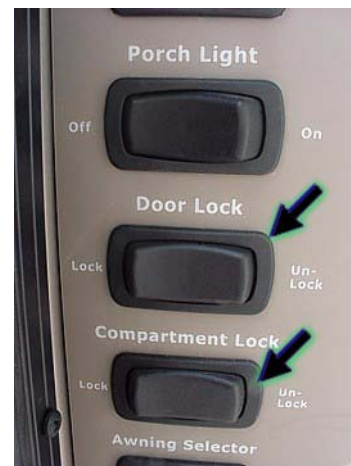
Power Door Locks on entry switch panel
