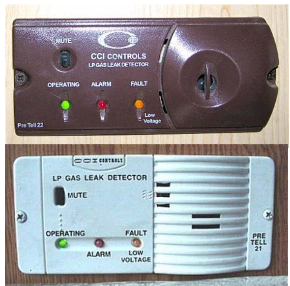
Propane Gas Leak Detectors (typical)
