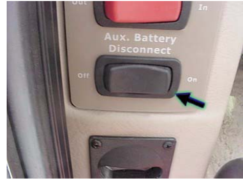
Aux. Battery Disconnect Switch (Near entrance door)
