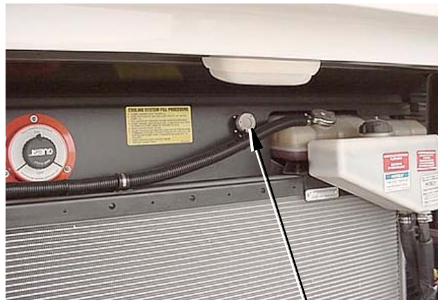
Diagnostic plug on rear engine compartment shroud
