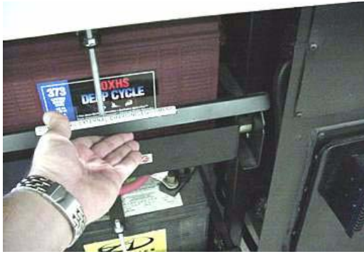
Lift Battery Tray Retainer Latches
