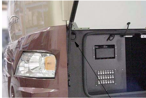
Hood Latch Location in 12-volt electrical compartment
