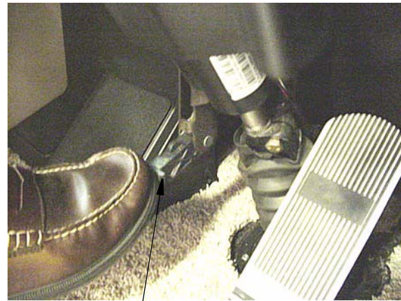
Press pedal at bottom of steering column to adjust steering wheel tilt or telescope
