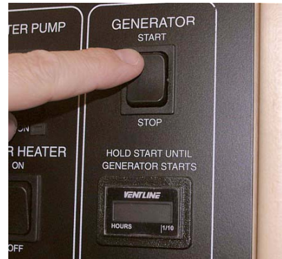
Generator Switch and Hourmeter
