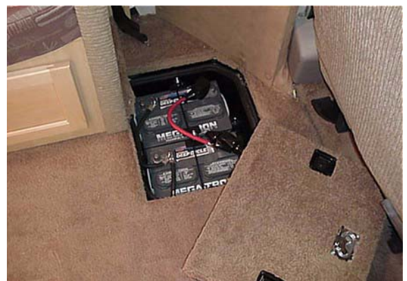
House Batteries in floor behind driver seat
