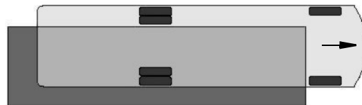
Weighing Right Rear Corner
