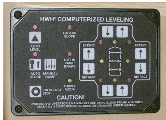
Leveling System Control Panel
