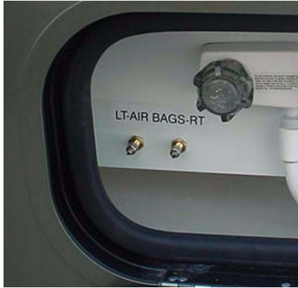
Rear Air Helper Spring Valves (located in water service center compartment)
