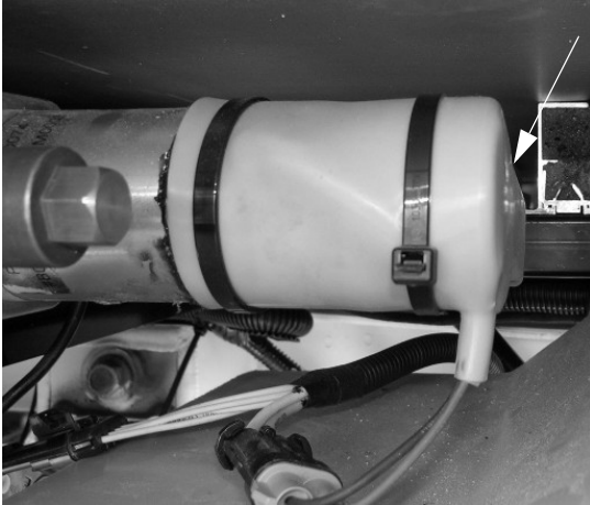
Electric Brake Lever (Located on back side of motor/gear assembly cylinder)
