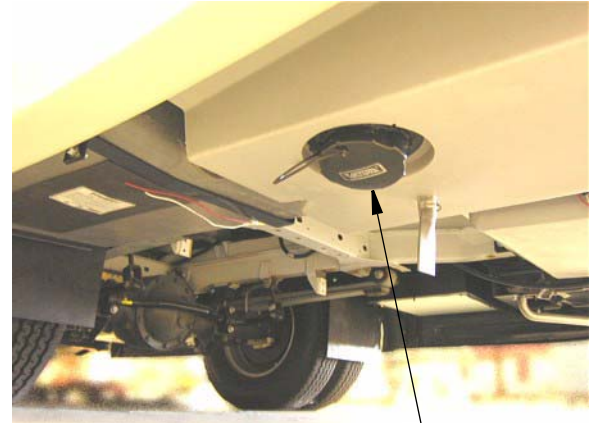
Sewage Drain Outlet on underside of water service compartment.
