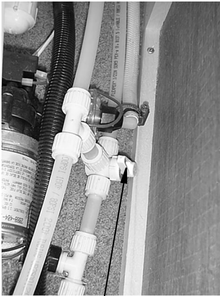
Waterline Drain Valve (Typical)
