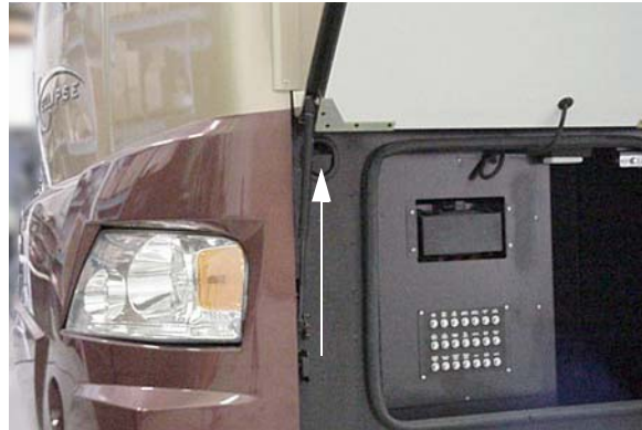
Hood Latch (Located in 12-volt electrical compartment) -Typical View
