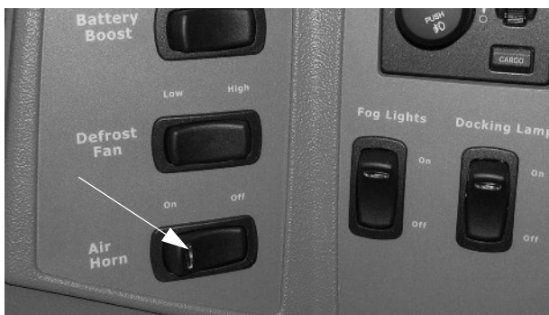
Air Horn Switch (Located on dash or driver side trim panel) -Typical View
