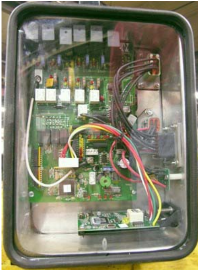
Hydraulic System Control Box (Located on pump beneath chassis near LH or RH front tire)
