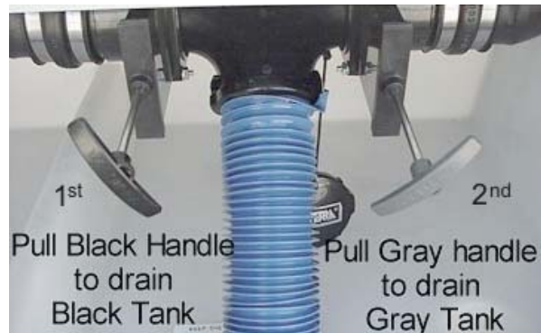
Holding Tank Valves (Typical)
