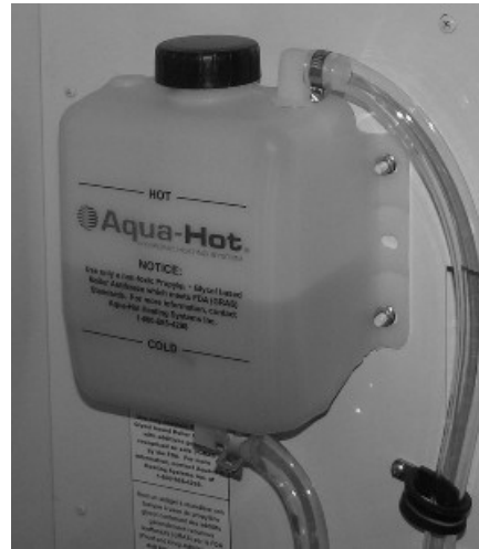
Expansion Fill Tank
