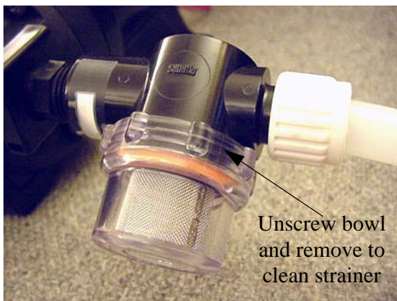
Water Pump Strainer -Typical View
