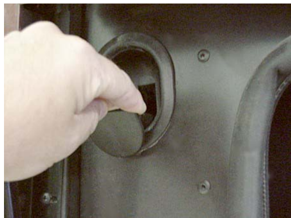
Hood Latch (Located in 12-volt electrical compartment) -Typical View
