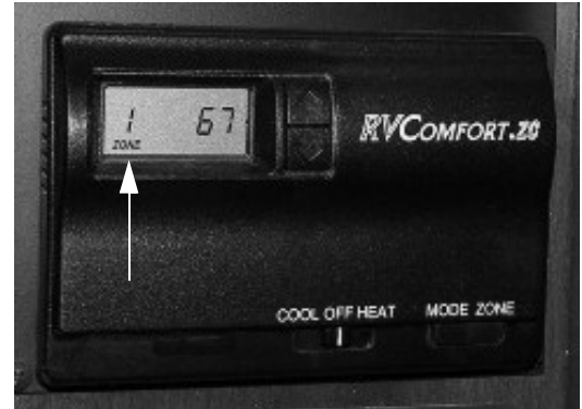
Zone 1 Operation (Living Area/Galley)
