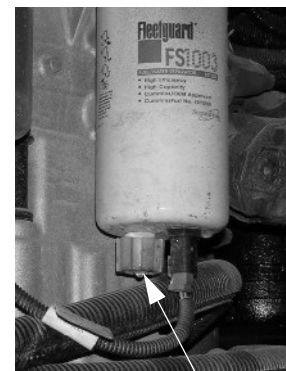
Detail of drain valve on bottom end of fuel/water separator
