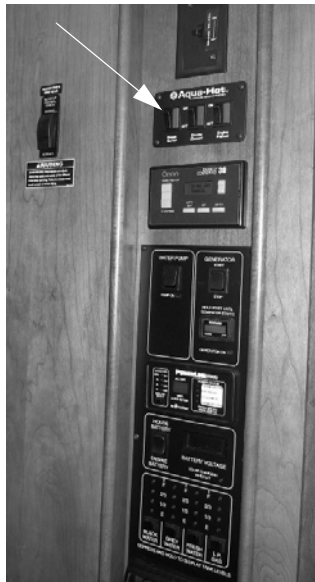
Hydronic Heating System Interior Control Switches (near OnePlace® monitor panel) -Typical View
