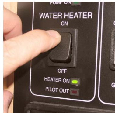
Gas Water Heater Switch (Located on monitor panel)
