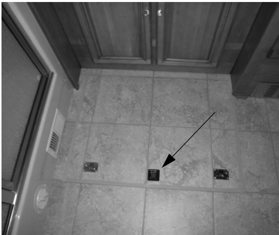
Rear Engine Access Cover Lock
