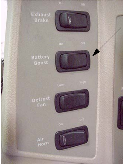
Battery Boost Switch (If chassis battery is discharged, press and hold while turning ignition key for emergency starting power) -Typical View
