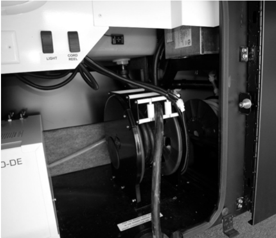
Power Cord Reel (Located inside an exterior compartment) -Typical View
