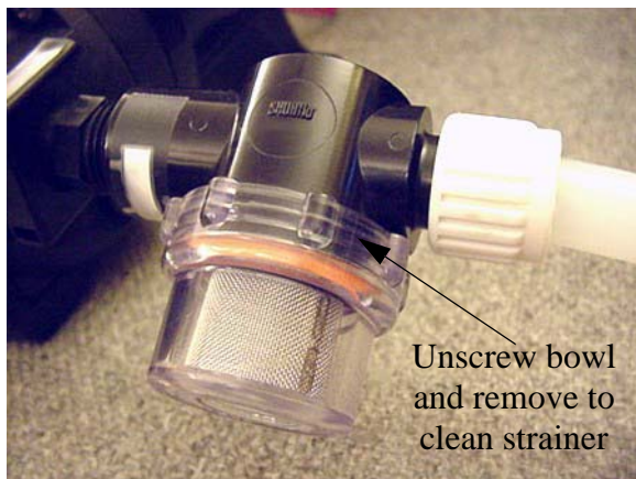
Water Pump Strainer -Typical View
