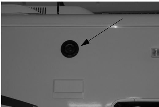
Exterior Speaker (Located below patio awning) -Typical View
