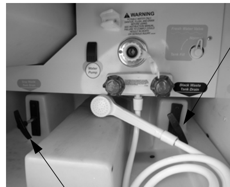
2nd - Pull Gray handle to drain Gray Water (sink/shower) tank – then close.
