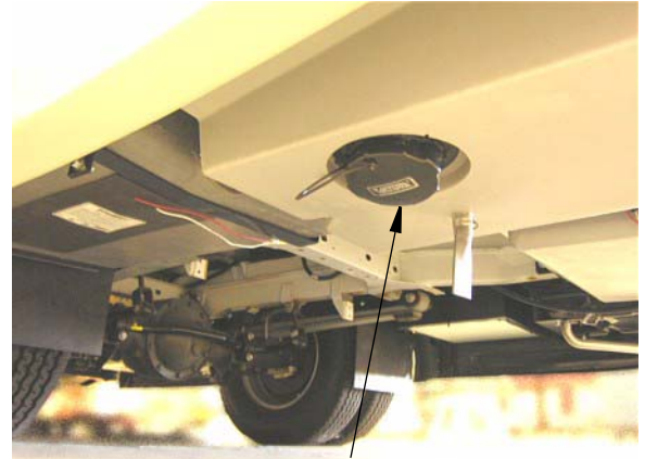
Sewage Drain Outlet (Located on the underside of water service compartment) -Typical View
