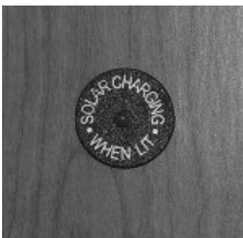
Solar Charging Indicator (Located near monitor panel)
