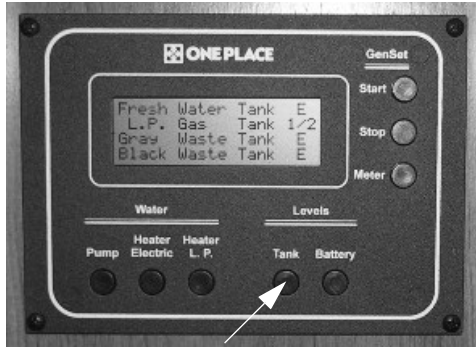
Tank Levels Switch
