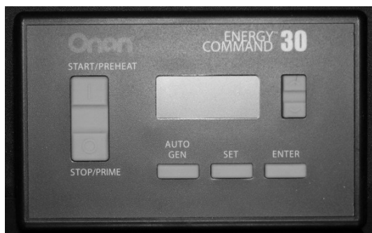
AGS Control Pad (Located near monitor panel)
