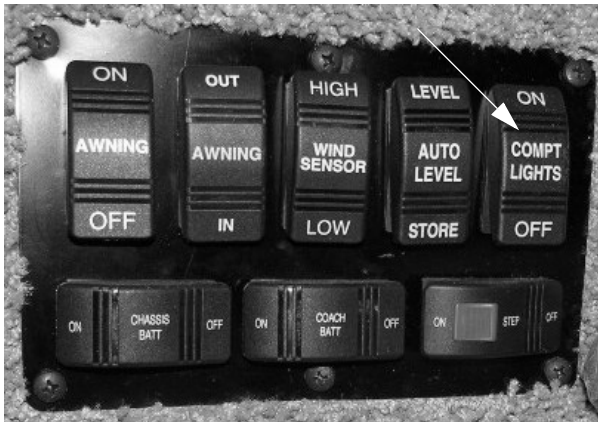
Compartment Lights Switch (Located near entrance door) -Typical View
