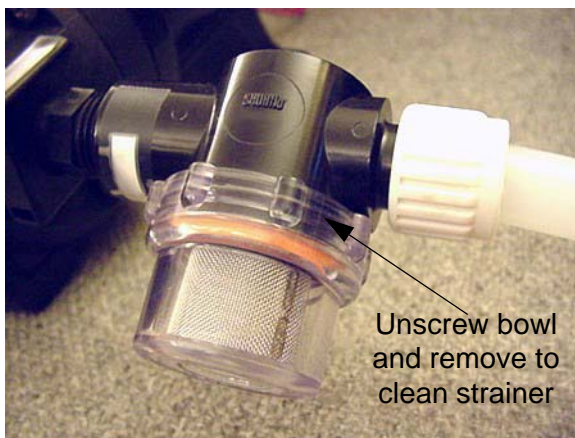
Water Pump Strainer -Typical View
