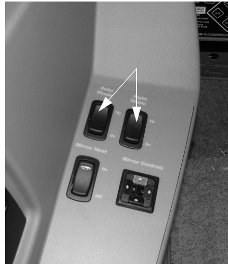
12-Volt Front Drop-Down Solar/ Night Shade Switches -Typical View
