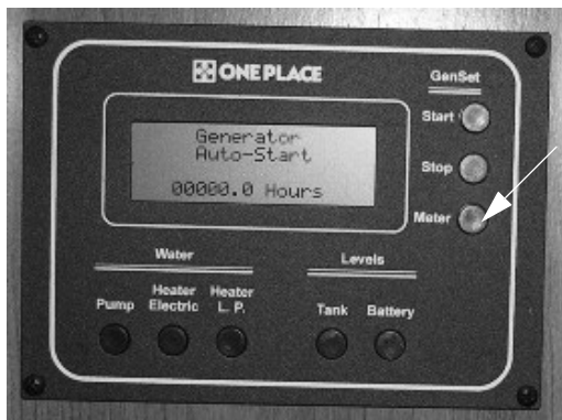
Generator Hourmeter Button -Typical View
