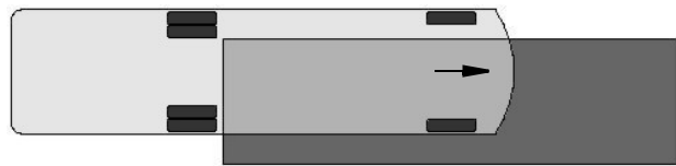
Weighing Right Front Corner
