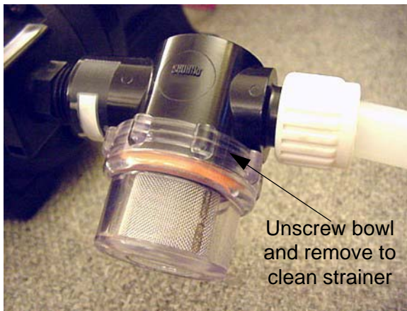
Water Pump Strainer -Typical View
