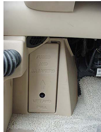
Automotive Fuse/Breaker Panel (Located beneath left end of dash)
