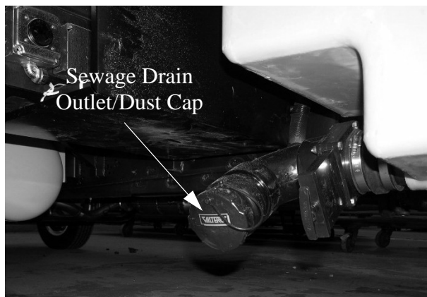
Sewage Drain Outlet (Located beneath coach on mid-driver side) -Typical View
