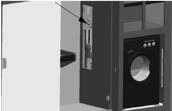
Water Supply Faucets (Located behind an access door within the rear wardrobe)
