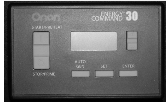
AGS Control Pad (Located near monitor panel)
