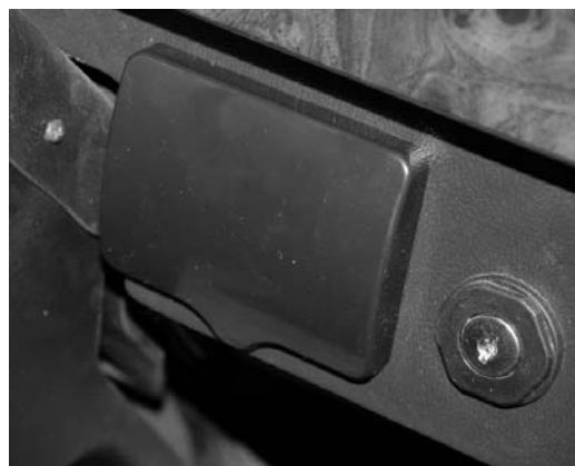
iPod Connection (Located on dash between steering wheel and key ignition) - Open cover to access iPod connection
