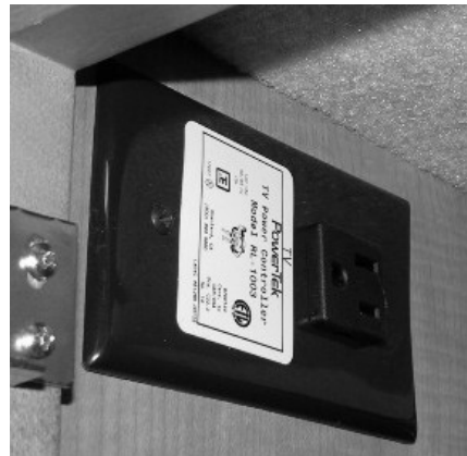
Front TV Ignition Switch Interlock -Typical View
