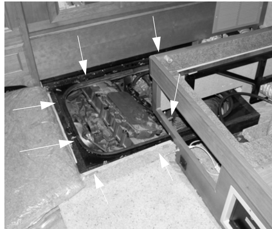
Step Cover Screw Locations -Typical installation shown
