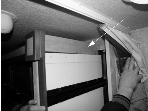
Slideout Travel Support -Typical installation shown
