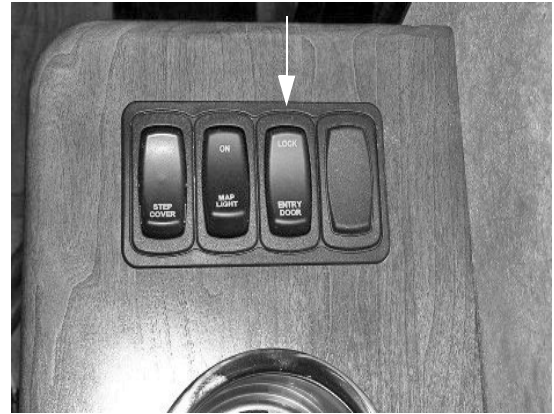
Power Door Locks - Entry Door (Located on passenger side armrest) -Typical View
