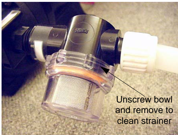
Water Pump Strainer -Typical View
