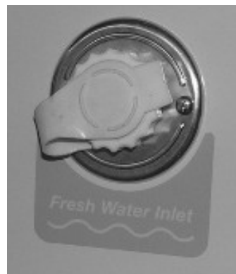
Fresh (City) Water Connection (Fresh Water Inlet)
