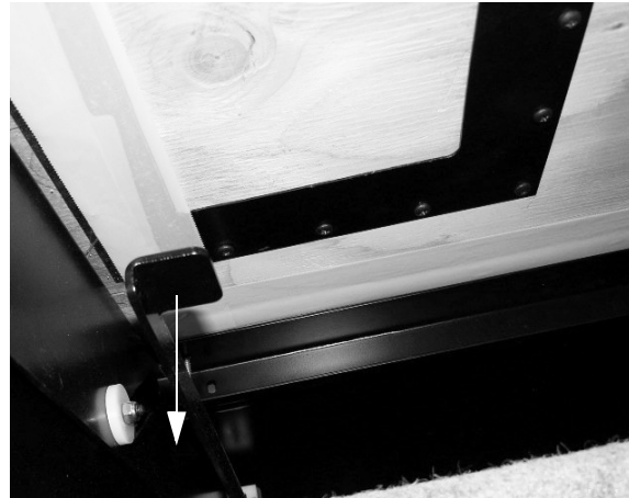
Emergency Retract Lever (Located underneath stepwell cover)
