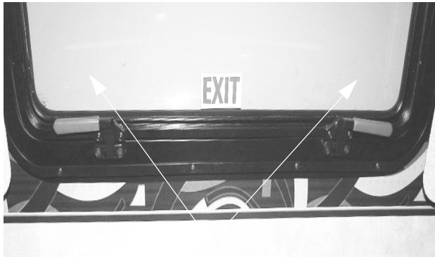
Escape Window (Lift latch handles upward to open)
