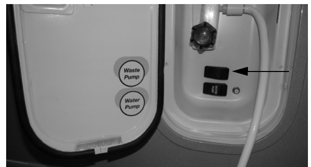
Waste Pump Switch (Located in water service center)
