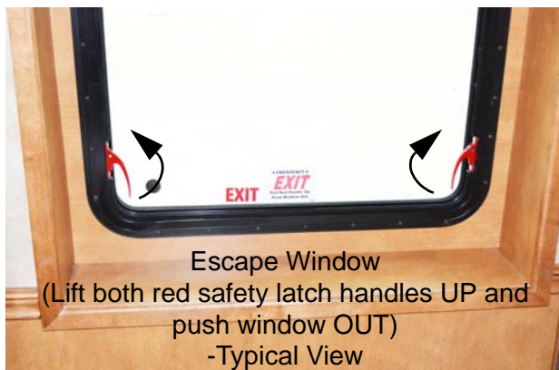
Escape Window (Lift both red safety latch handles UP and push window OUT) -Typical View
