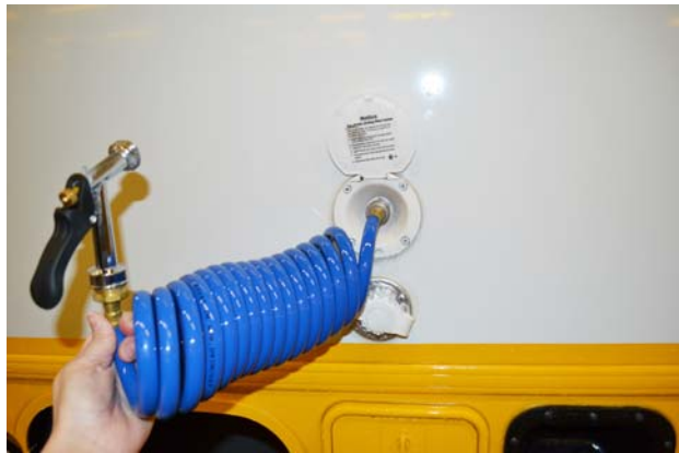
Exterior Shower/Wash Station -Typical View
