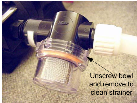
Water Pump Strainer -Typical View
