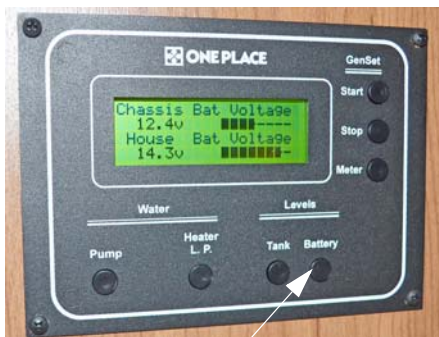
Battery Levels Switch
