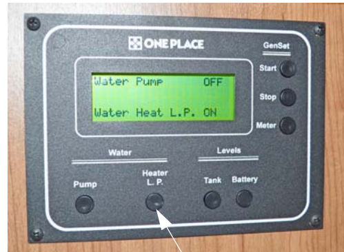
LP Gas Water Heater Switch
