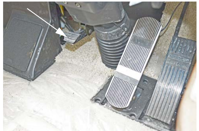
Press pedal down to adjust steering wheel tilt or telescope
