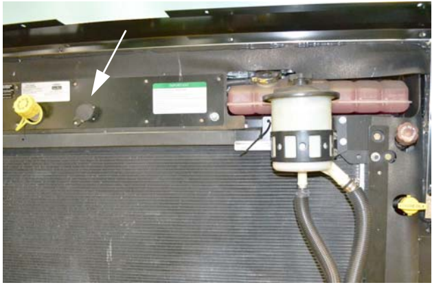
Diagnostic Plug (Located on rear engine compartment shroud) -Typical View
