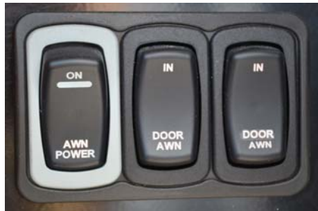
Awning Control Switches (Located near entrance door) -Typical View
