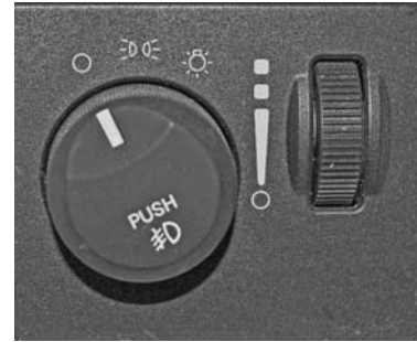
Headlight Switch (Located on left side of dash) -Typical View
