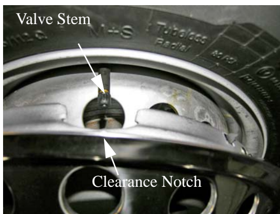
Valve Stem Clearance Notch aligned to Valve Stem
