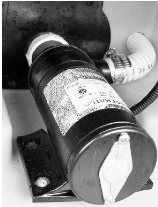
Waste Pump (Located beneath coach) -Typical View
