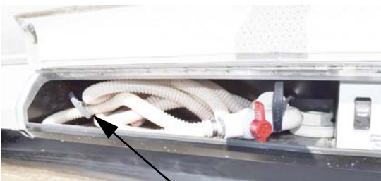
Gray Waste Tank Drain Valve (Located in water service center)
