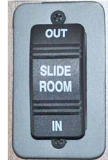
Slideout Switch -Typical View
