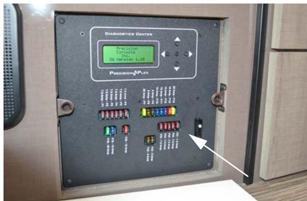
House 12-Volt Fuses (Model 70A and 70X) -Typical View
