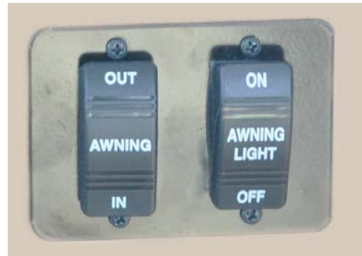
Power Awning and Awning Light Switch (Located at front of galley) -Typical View
