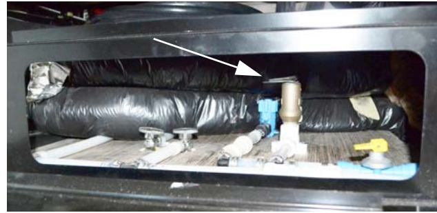
Pressure Temperature Relief Valve • Lift handle only when water heater is cold (See “Water System Drain Valve Locations” chart at the end of this section for location on your model) *Model 70X shown
