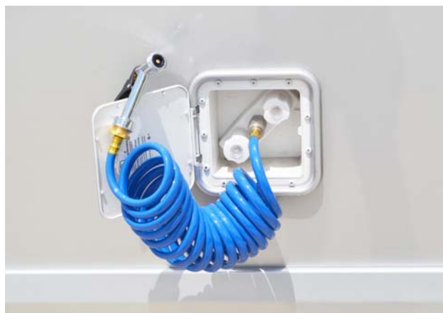
Exterior Shower/Wash Station (Typical)
