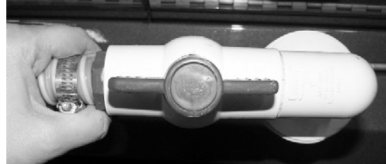
Sewage Drain Hose Valve
