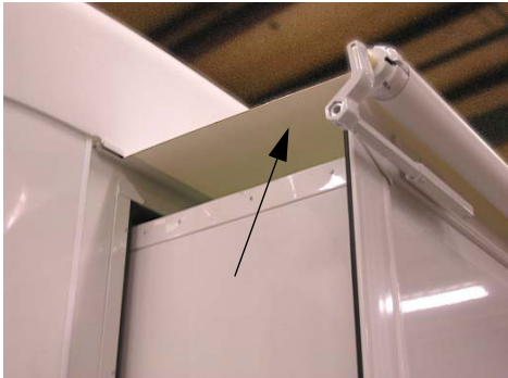
Slideout Cover-Awning -Typical View
