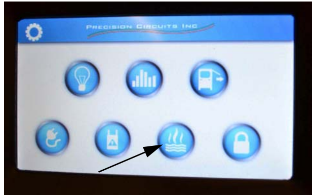
Water Pump Switch
