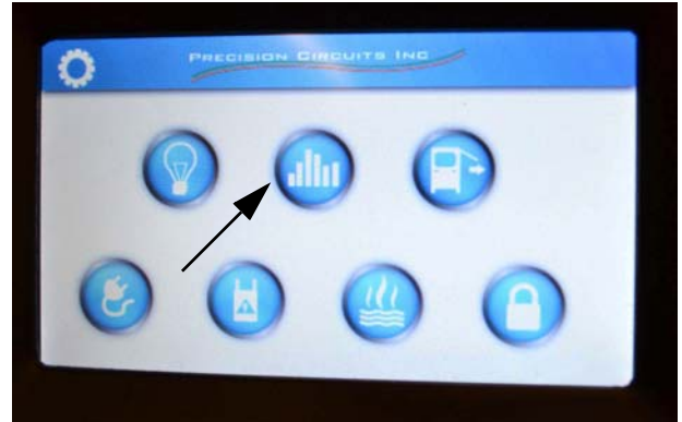
Levels Test Switch
