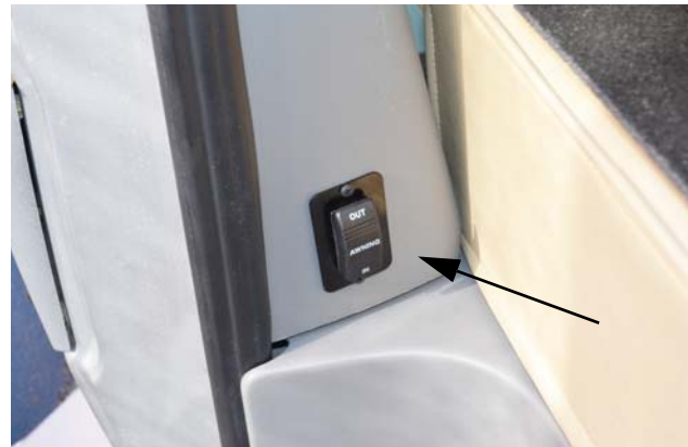
Second Power Awning Switch (Located near right side of passenger seat) -Typical View
