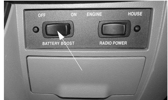
Battery Boost Switch (Located on dash)
