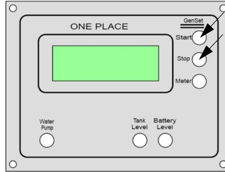
Generator Start/Stop Buttons (Located on monitor panel) -Typical View
