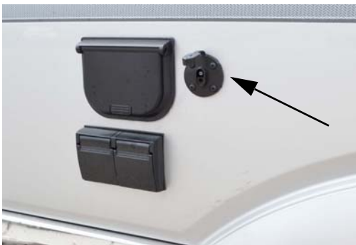
Single Solar Port (Located on an exterior sidewall) -Typical View
