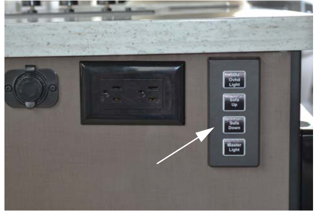
Sofa Up and Sofa Down Switches (located on cabinet wall ahead of the couch)
