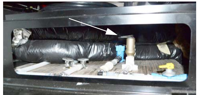
Pressure Temperature Relief Valve • Lift handle only when water heater is cold (See “Water System Drain Valve Locations” chart at the end of this section for location on your model) *Model 70X shown
