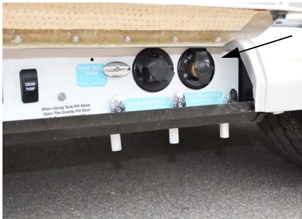
Black Waste Tank Flush Inlet (Located in water center compartment) -Typical View
