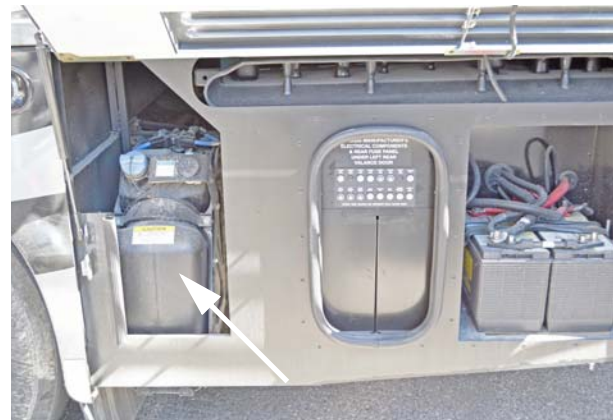
Diesel Exhaust Fluid Fill Tank *with Rear Radiator (Located in driver side compartment behind the rear wheel) -Typical View
