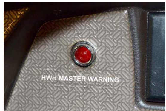
HWH® Master Warning Light (Located on dash)
