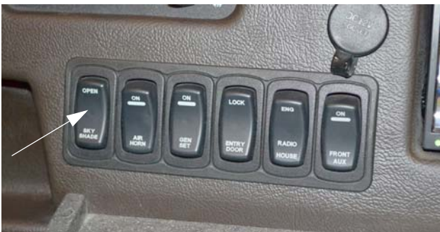
Skylight Shade Control Switch (Located on dash)
