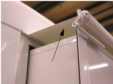
Slideout Cover-Awning -Typical View
