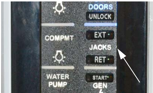
Auto Level Remote Switch (Located near entrance door and/or inside exterior service center) -Typical View
