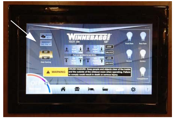
Hydronic Heating System Interior Control Switches (Located on touch tablet “Exterior” screen)
