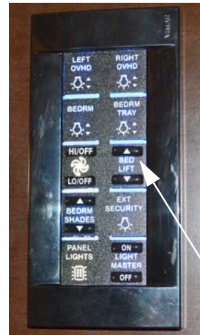
Power Lift/Lower Control Switch (Located on overhead cabinet above bed) –Typical View
