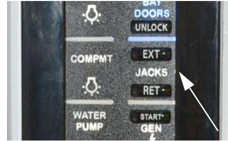
Auto Level Remote Switch (Located near entrance door and/or inside exterior service center)
