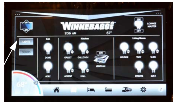
Power Roof Ventilator Switch (Located on touch tablet “Lounge” screen) -If Equipped
