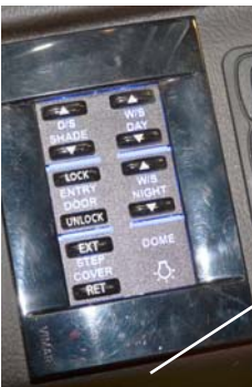
Step Cover Switch (Located on driver side trim panel) -Typical View
