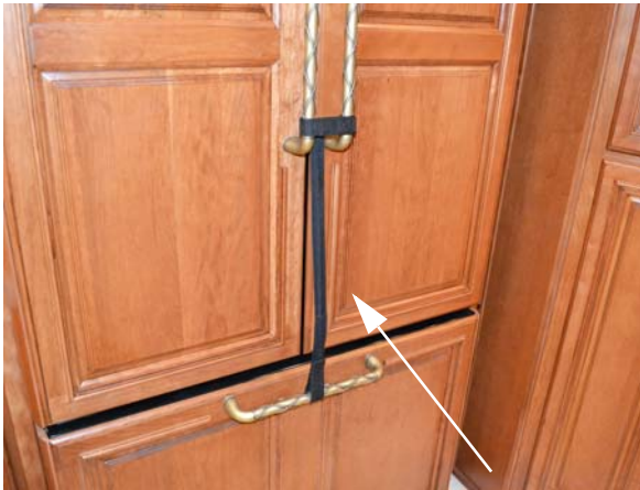
Refrigerator/Freezer Travel Latch (locked position) -Typical View
