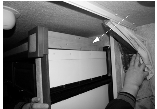
Slideout Travel Support -Typical installation shown
