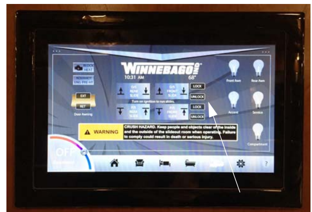
Slideout Room Travel Lock (Located on touch tablet “Exterior” screen)
