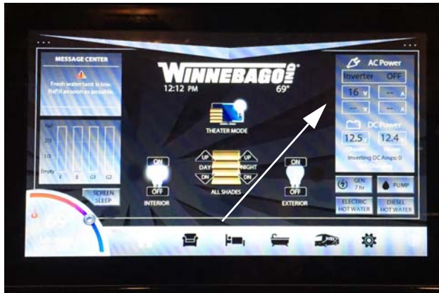
Inverter Status (Located on touch tablet “Home” screen) -If Equipped
