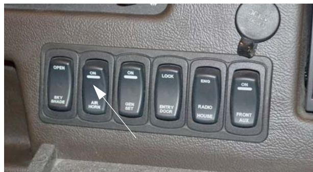
Air Horn Switch (Located on dash or driver side trim panel) -Typical View
