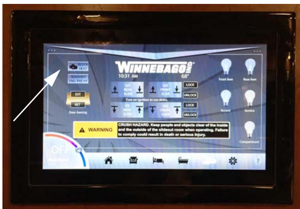
Diesel Engine Heater Switch (Located on touch tablet “Exterior” screen) Tap to turn Block Heater on/off • White text indicates ON • Black text indicates OFF -If Equipped
