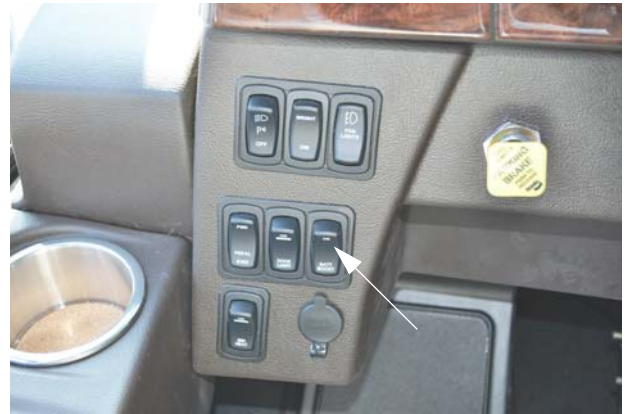
Battery Boost Switch (Located on dash)
