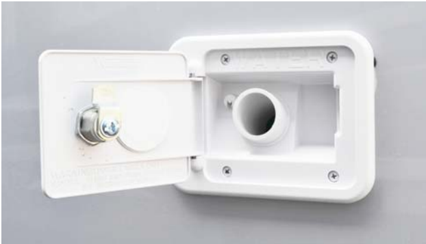
Water Tank Gravity Fill -Typical View
